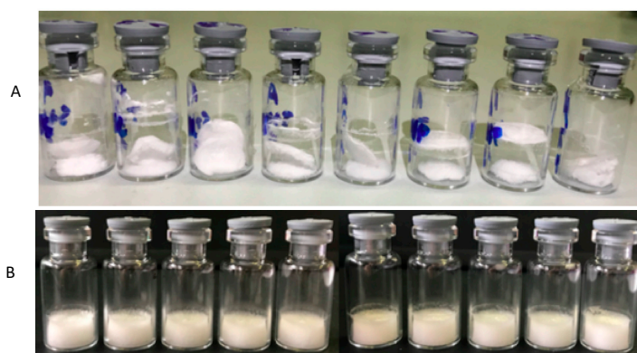
Figure 4. Cakes obtained after lyophilization of formulations with 1% v/v ethanol content (A) and 0.1% v/v ethanol content (B): Figure 4A clearly evidences the phenomenon of “product ejection”.
