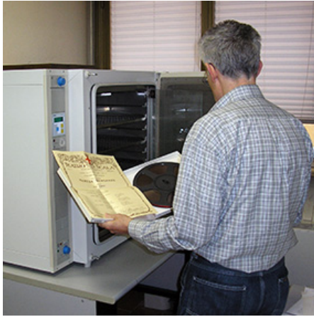
Fig. 2. The Heraeus UT6200 oven used to thermally pretreat magnetic tapes.
