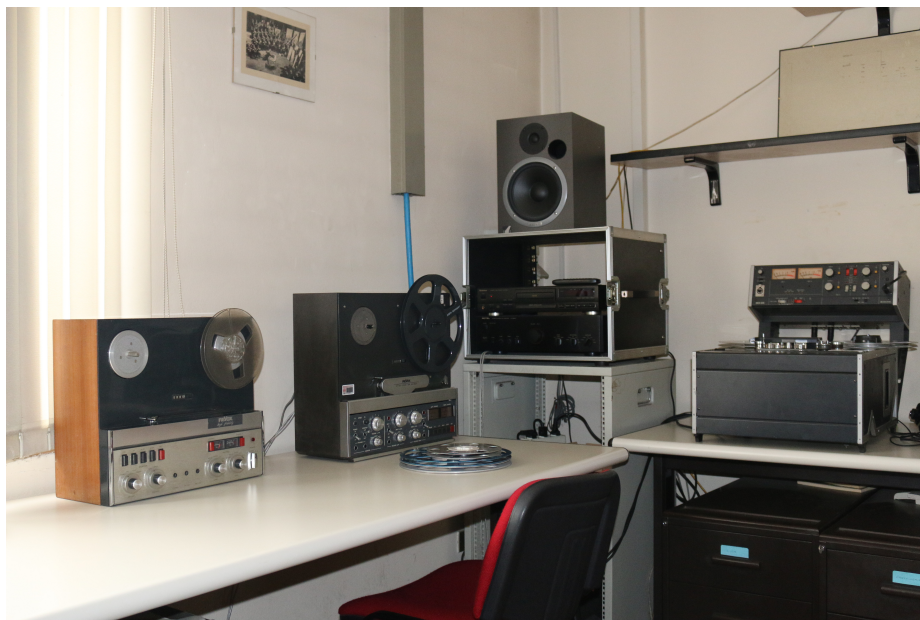
Fig. 1. Devices for open-reel magnetic tapes in the LIM digitization studio: from left to right, Revox A77, Revox B77 MKII and Otari MX-55.
