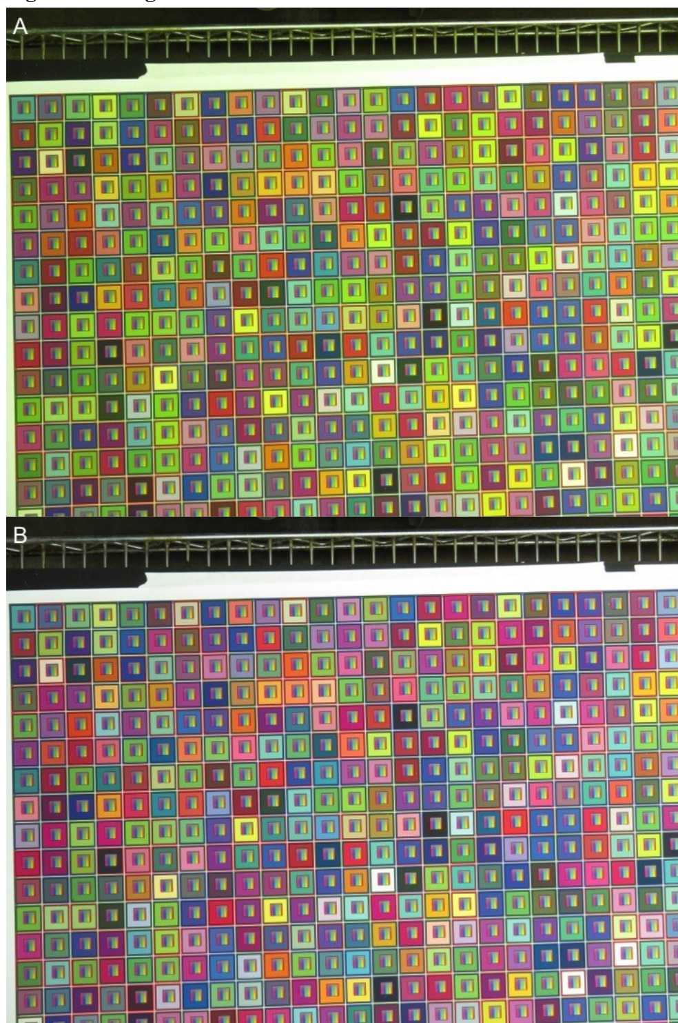
A) The image before the image color correction. The green tone of the image was due to shelf illumination. B) The image after the color correction shows that the green tone was removed.
