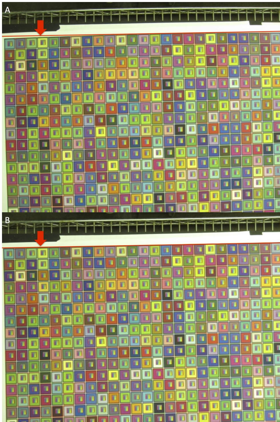
A) The image before the image optical distortion correction. The red reference line on the top shows the curvature of the edge of the color grid. B) The image after the image optical distortion correction. The edge of the color grid shows straight comparing the red reference line.
