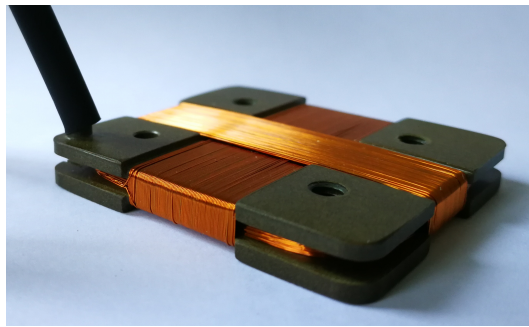
Figure 12. Prototype of a three axis pick-up magnetic probe for RFX-mod2 (37 × 42 × 5 mm).
