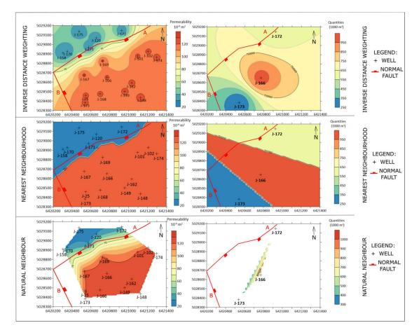
**Figure 3.** Results of inverse distance weighting (IDW), nearest neighbourhood (NN) and natural neighbourhood (NaN) methods (from top to bottom) of the permeability (left) and injected volumes (right) in the "K" reservoir [41].
