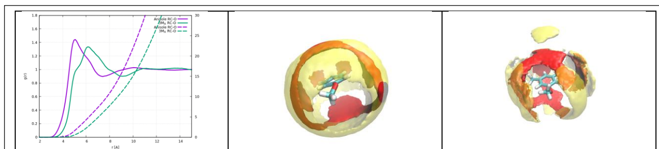
Figure 8. Spatial distribution of oxygen atom surrounding reference anisole and 3M_A compounds. (Left) Pair distribution function and coordination numbers of RC-O correlations for the two compounds. Spatial distribution function of oxygen atom surrounding reference anisole (center) and 3M_A (right). Distribution isovalues refer approximately to half of the maximum amplitude. a) anisole, red (layer between 0 and 5.5 Å), transparent yellow (layer between 5.5 and 7.4 Å); b) 3M_A, red (layer between 0 and 5.5 Å), transparent yellow (layer between 5.5 and 9.2 Å).
