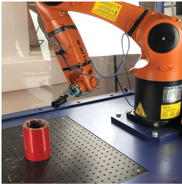
Fig. 3: Industrial machine vision camera attached to the end effector of KUKA AGILUS.
