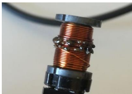
Fig. 16. Photograph of an inductor damaged by thermal collapse.
