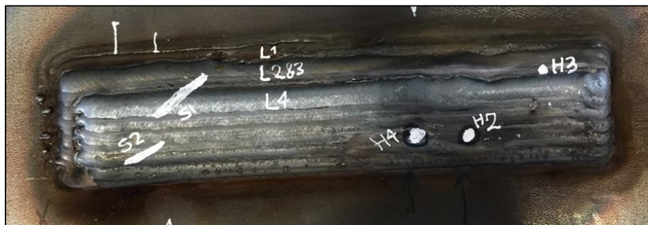
FIGURE 6. Defects successfully embedded inside the sample
