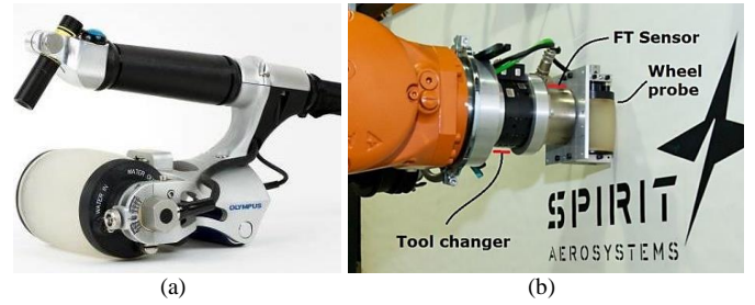
Fig. 2. RollerFORM® in its original configuration (a) and mounted onto the robot through a support (b)
