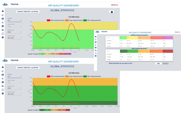
Fig. 6. Two year views for CO in 2020: the bottom uses ARPAE scale and the top EEA scale. The figure shows also the setting view where scales can be modified.
