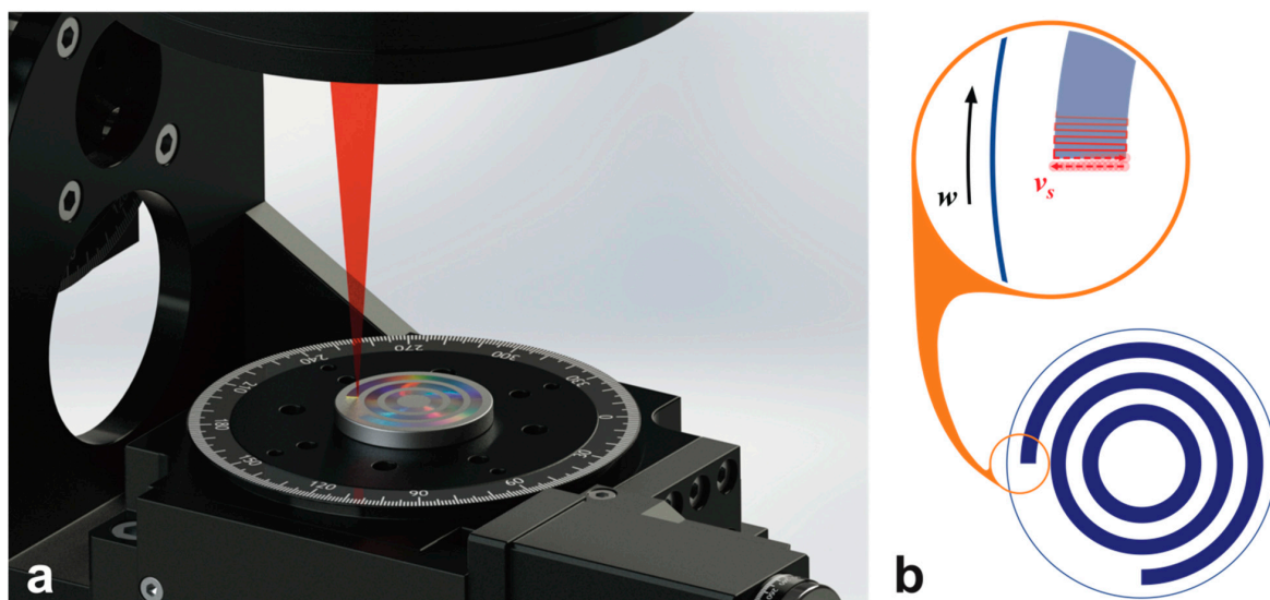
Figure 1. (a) Schematic of the laser treatment as a laser beam is scanned over a sample. (b) Details of laser patterning strategy: the laser beam is moving forth and back, while the sample is rotating by angular stage.
