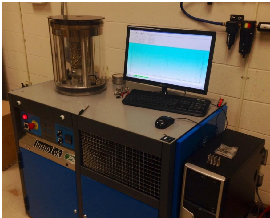
Figure 4.10 Creep Test on HMA Samples (Saghebfar 2014)
