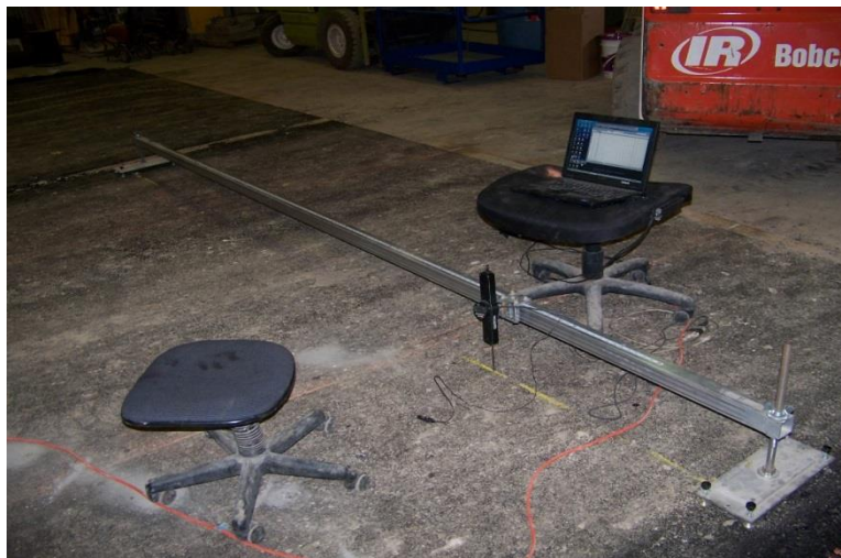
Figure 3.6 Transverse Profiler at CISL (Saghebfar 2014)
