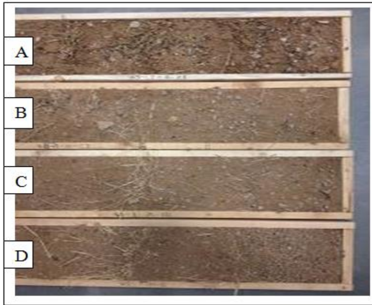
Figure 3-20. Surface conditions of wind tunnel trays from curve outside section trafficked by wheeled vehicle at White Sands Missile Range (sandy loam): (A) undisturbed, (B) 10 passes, (C) 25 passes, and (D) 50 passes.
