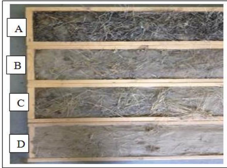
Figure 3-18. Surface conditions of wind tunnel trays from curve outside section trafficked by light-wheeled vehicle at Yakima Training Center (sandy loam): (A) undisturbed, (B) 10 passes, (C) 25 passes, and (D) 50 passes.
