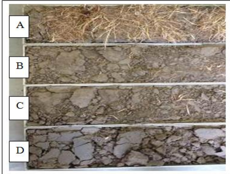
Figure 3-16. Surface conditions of wind tunnel trays from the curve outside section trafficked by treated tracked vehicle at Fort Riley (silt loam): (A) undisturbed, (B) 1 pass, (C) 5 passes, and (D) 10 passes.
