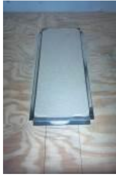
Figure 3-22. Metal frame used to place sand abrader on the tunnel floor.
