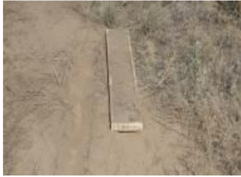
Figure 3-5. Wind tunnel tray sample extracted from Yakima Training Center, WA.
