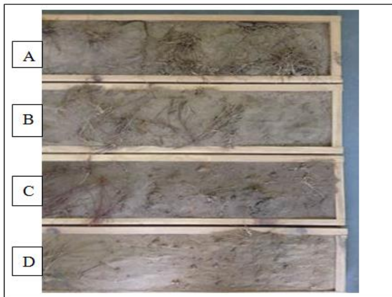
Figure 3-17. Surface conditions of wind tunnel trays from curve outside section trafficked by wheeled vehicle at Fort Benning (loamy sand): (A) undisturbed, (B) 10 passes, (C) 25 passes, and (D) 50 passes.
