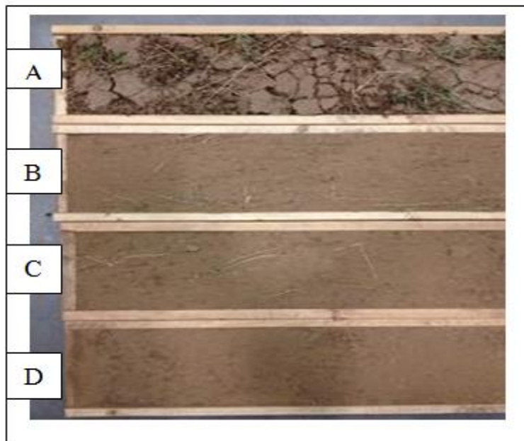
Figure 3-19. Surface conditions of wind tunnel trays from curve outside section trafficked by wheeled vehicle at White Sand Missile Range (loam): (A) undisturbed, (B) 10 passes, (C) 25 passes, and (D) 50 passes.
