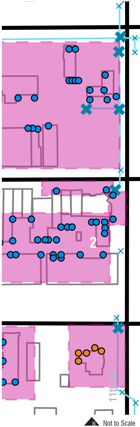
Figure 02. Downspout Examples some downspouts dump stormwater beyond permeable surface (Krehbiel 2014)
