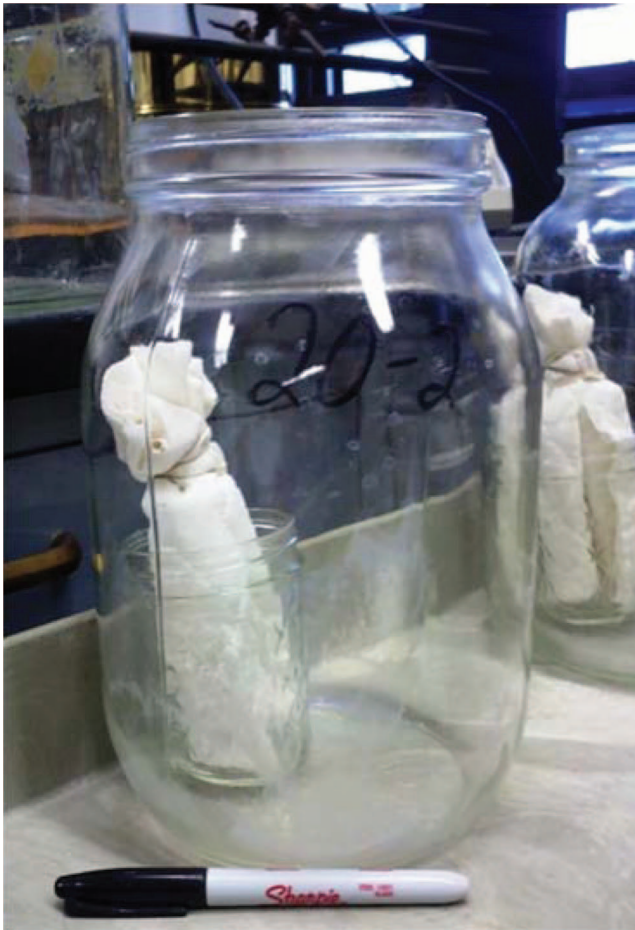
Fig. 2. A group of vials containing bed bug eggs that were wrapped in bedding material before fumigation to simulate a habitat for bed bugs that might be subject to fumigation with SF. Screw-on lid with injection port not shown. (Online figure in color.)
