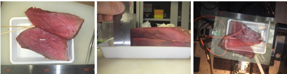
FIGURE 7.10: Beef experiment II: (Left) A cylindrical fluorescence target was inserted in the beef meat. (Middle) The cylinder was embedded at depth about x_3 = 10 mm. (Right) Scanned on the meat surface to obtain the boundary measurements.
