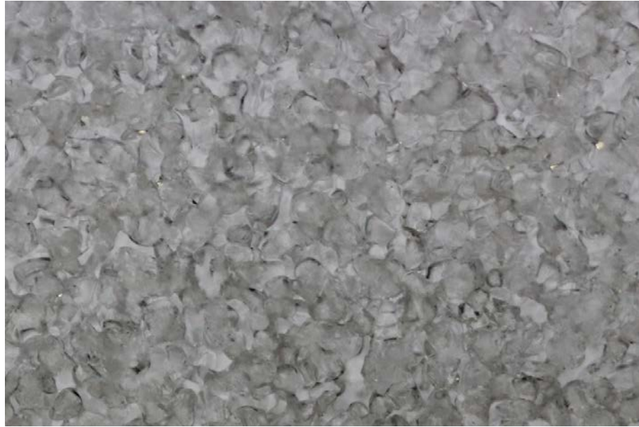
Figure 11S. Photograph of the sintered glass in the filter holder.
