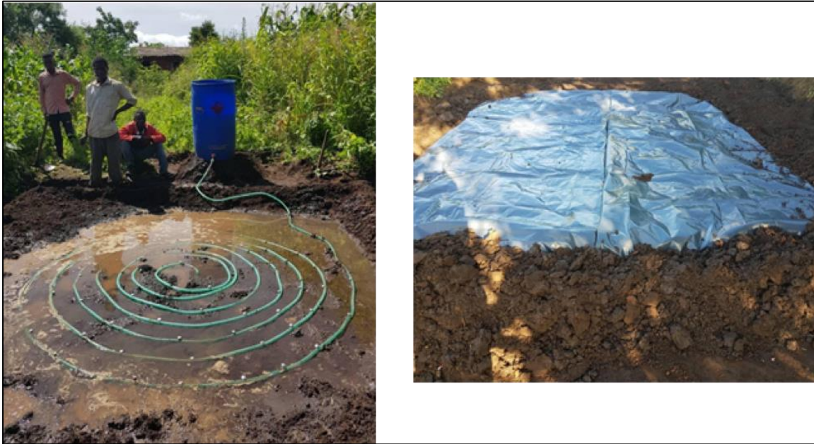
Figure 34. Two-stage process of determining the soil moisture at field capacity for APSIM model parameterization. Firstly, an area of at least 3 m diameter is wetted to saturation point to an entire root zone depth (Left photo). The wetted area is then covered by a plastic sheet for a period of two weeks (Right photo). Soil water above field capacity is lost through gravitational drainage. Moisture content in soils sampled in the wetted zone after 2 weeks is a good estimate of field capacity. Photo credit: Regis Chikowo/IITA.
