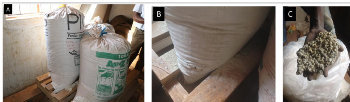
Figure 22. A case of technology failure: (A) AgroZ bag (single liner) and PICS bag (double liner) placed side by side; (B) insect holes on the outer polypropylene bag of the PICS bag and grain powder around it; (C) caked damaged grain from the PICS bag. The ferocious larger grain borer was identified in this particular store (Changarawe Village), and also in some other farmers' stores with an overall prevalence rate of 8.5%. The AgroZ bag outperformed the double liner PICS bags at this farmer's store. Photo credit: Christopher Mutungi/IITA.
