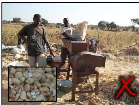
Poorly calibrated threshers damage kernels (see inset).
