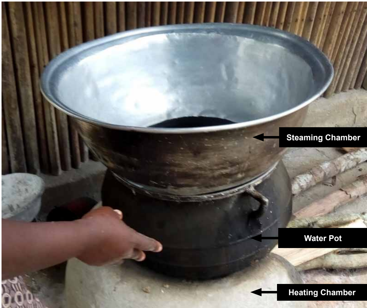
Plate 10. Components of the traditional steamer.
