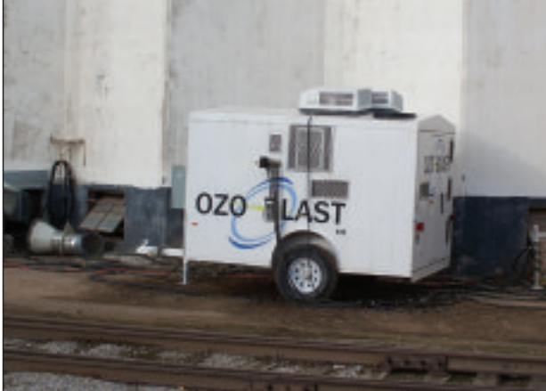
Above is a mobile unit that can generate ozone gas on site using electricity. Photo supplied by O3Co.
