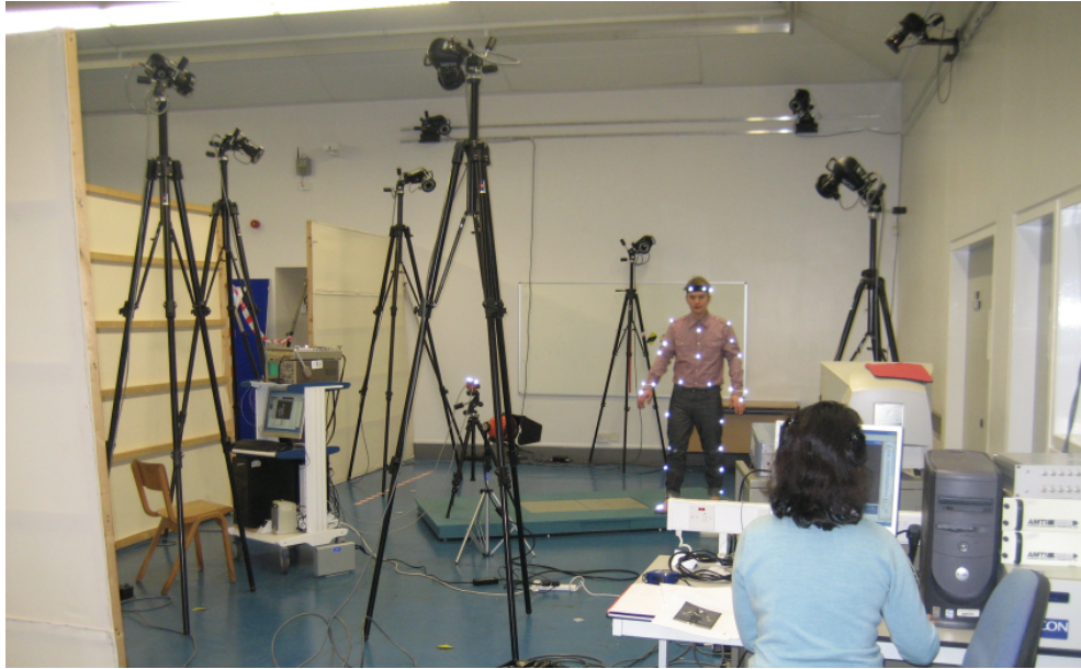
FIGURE 3.22: Motion capture lab. Retro-reflective markers on the subject’s body are returning light from the camera’s flash bulb.
