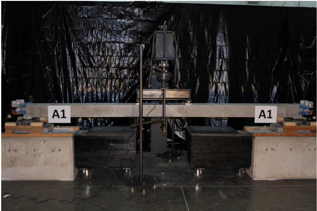
Figure 11.4 Beam A1 Setup for Simple Quality Assurance Test for Strand Bond
