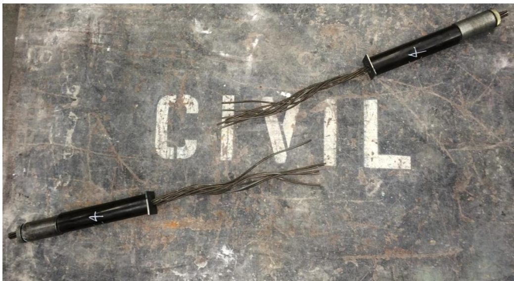
Figure 10.1 Ultimate Tensile Strength of Strand Test Specimen after Failure
