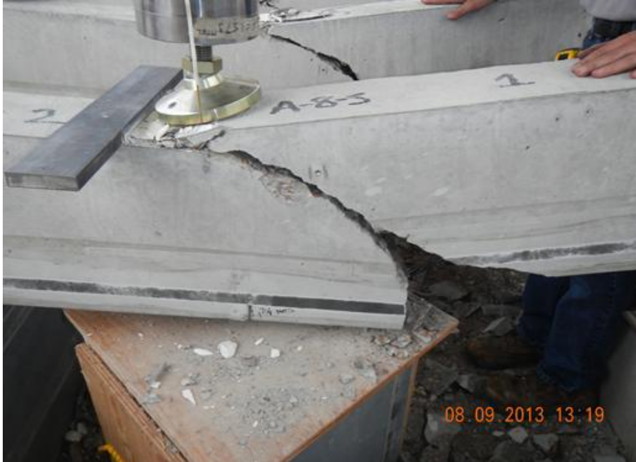
Figure H.54 Beam End A8-S Failure
