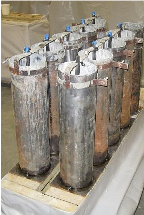
Figure 4.2 Specimen Setup (Polydorou, Riding, Peterman, & Murray, 2013)
