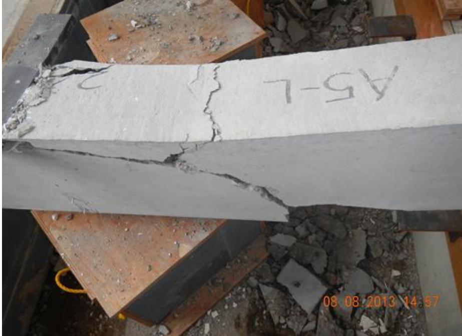
Figure H.15 Beam End A5-L Failure
