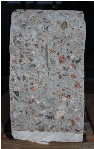
Figure 9.9 Saw Cut on Bottom Surface of Beam
