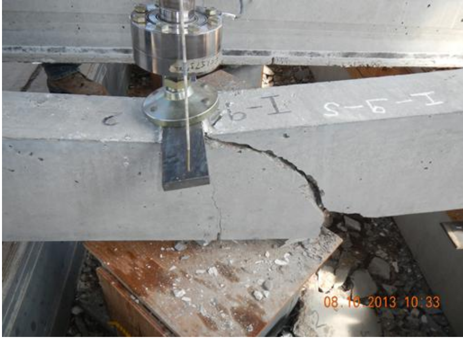
Figure H.176 Beam End I9-S Failure
