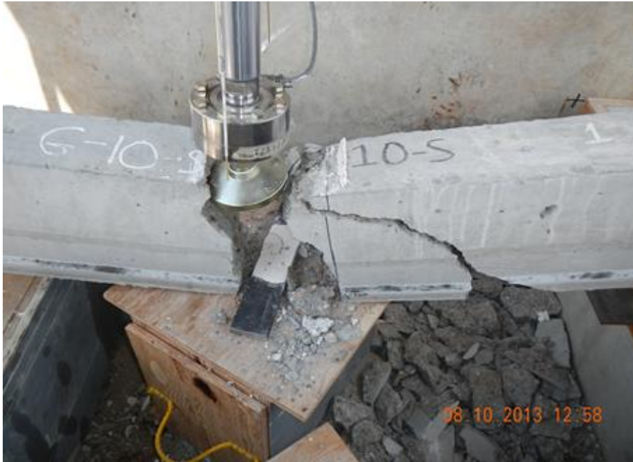
Figure H.119 Beam End G10-S Failure
