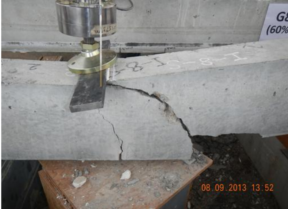
Figure H.113 Beam End G8-S Failure
