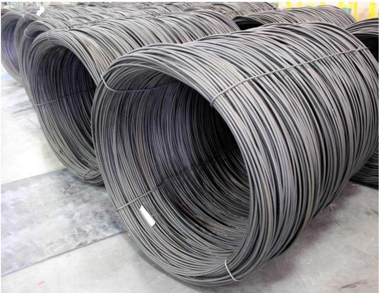
Figure 2.2 Raw Steel Coils used for Prestressing Strand Manufacturing
