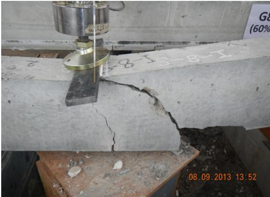
Figure H.173 Beam End I8-S Failure
