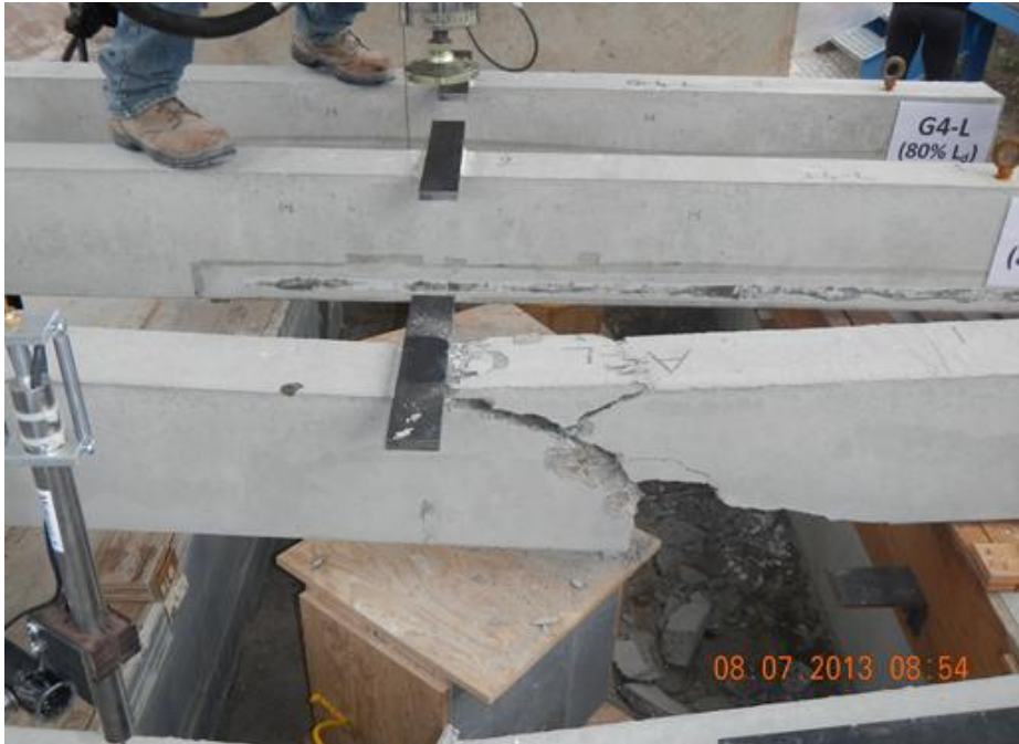
Figure H.12 Beam End A4-L Failure
