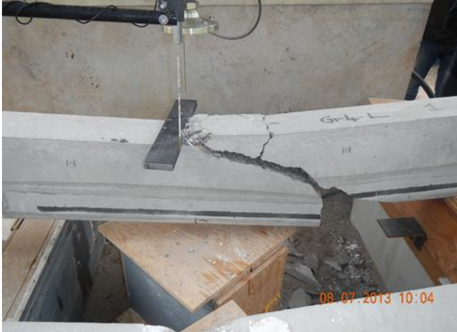
Figure H.71 Beam End G4-L Failure
