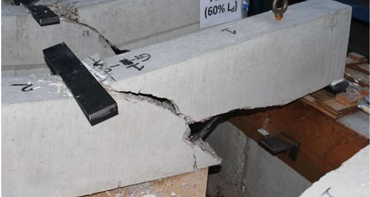
Figure H.92 Beam End G1-S Failure
