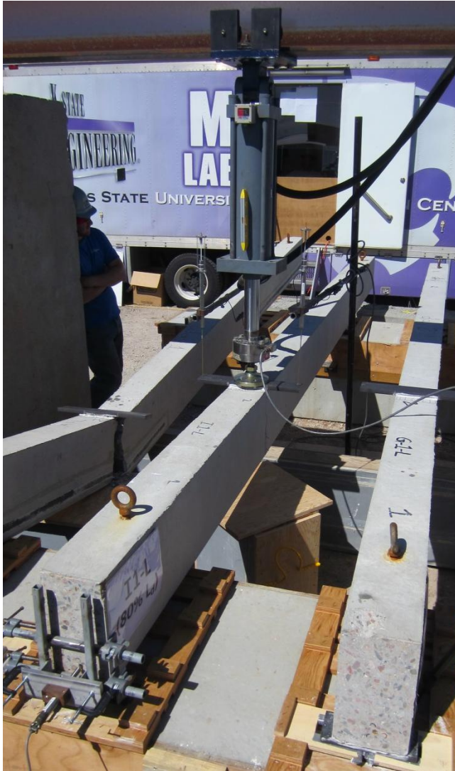
Figure 9.17 Beam Testing Setup: Load Cell, Load Point LVDTs, End Slip LVDT
