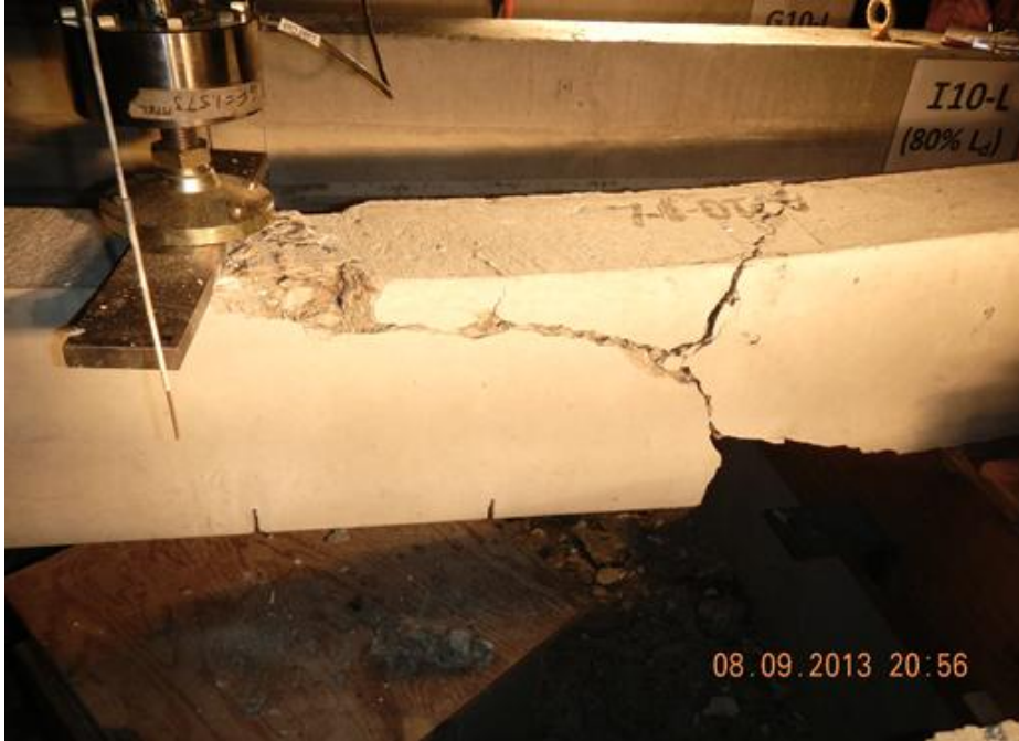
Figure H.30 Beam End A10-L Failure
