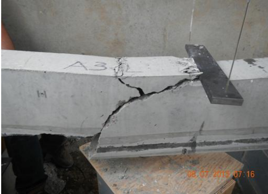
Figure H.9 Beam End A3-L Failure
