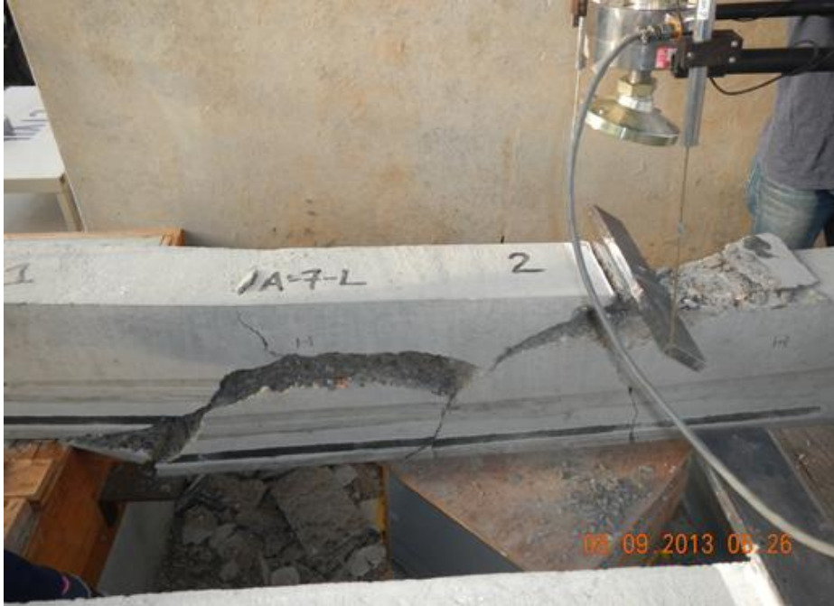
Figure H.21 Beam End A7-L Failure
