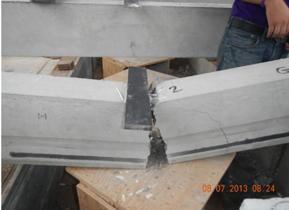
Figure H.68 Beam End G3-L Failure
