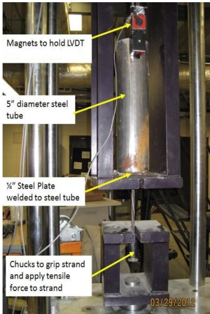
Figure 4.3 Tensile Testing Frame (Polydorou, Riding, Peterman, & Murray, 2013)
