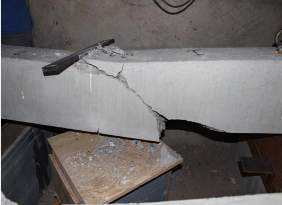
Figure H.95 Beam End G2-S Failure
