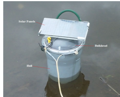
Figure 8. Buoy station prototype field test.
