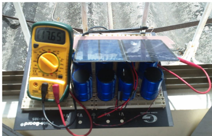
Figure 7. Power supply test, ultracapacitor stack voltage level of 17.65 V.
