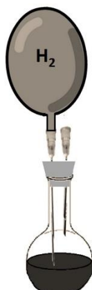
Figure 3.13. Molecular hydrogen experimental set-up scheme.
