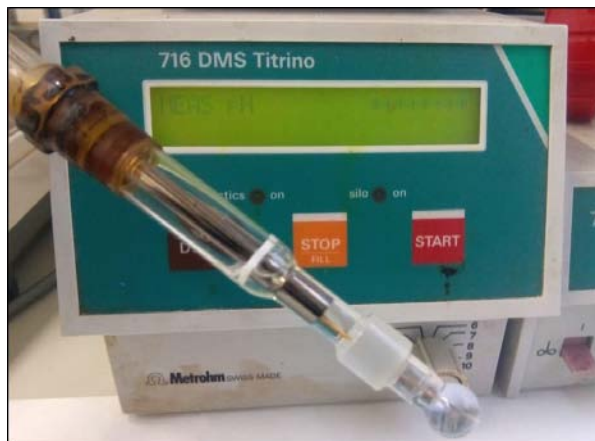
Figure 3.2. pHmeter picture and Solvotrode electrode.
