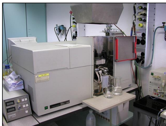
Figure 3.6. Perkin–Elmer flame atomic absorption spectrophotometer.
