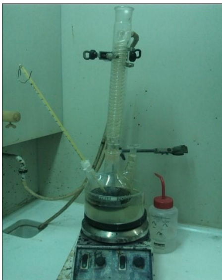
Figure 3.11. Picture of experimental set-up for assessment of the catalytic upgrading process.
