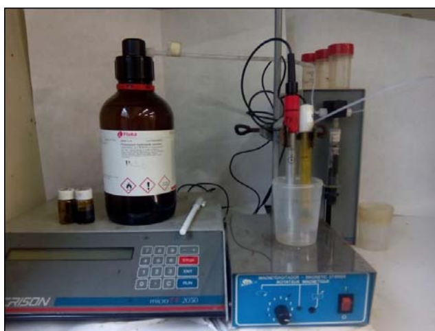
Figure 3.3. Crison micro TT 2050 potentiometer for Total Acid Number titration.
