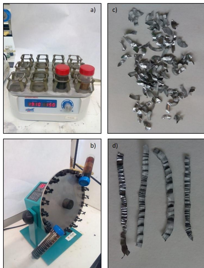
Figure 3.15. Picture of the shakers used and the pieces of Zn: orbital shaker with horizontal circular movements (a); Vertical rotation shaker (b); Zn pieces of 2.5 x 8 mm (c); Zn pieces of 2.5 x 80 mm.
