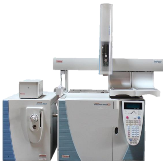
Figure 3.1. Gas Chromatograph TRACE GC ULTRA coupled to a DSQ II Mass Spectrometer and a TRIPLUS AS autosample from ThermoFisher Scientific.
