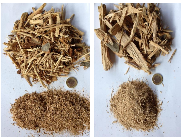
Figure 4.3. Comparison between raw and grinded biomass: almond pruning waste (a); olive pruning waste (b).
