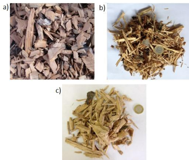
Figure 4.1. Pictures of potential valuable raw biomasses: cherry pruning waste (a); almond pruning waste (b); olive pruning waste (c).
