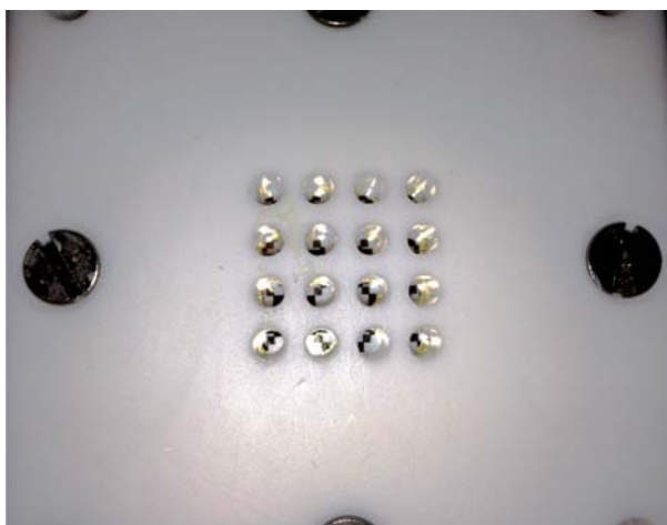
Figure 9.9: Assembled molds and support layer prior to the micropillar array fabrication. Notice that each thermoresistor is centered of a hole.
