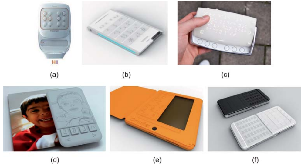
Figure 1.7: Recent proposals for the integration of Braille into new technologies: a) Touch Messenger Braille mobile phone from Samsung Electronics, 2006 [57]; b) Tactility Toshiba mobile phone designed by Siwei Liu, 2009 [58]; c) Squibble Portable Braille Interface designed by Andrew Mitchell, 2009[59]; d) Touchscreen Braille phone, designed by Sumit Dagar, 2011 [60]; e) Omnifer case designed by J. D’Alessandro from Auburn University [61]; and f) DrawBraille Mobile Phone designed by Shikun Sun from Sheffield Hallam University, 2012 [62].
