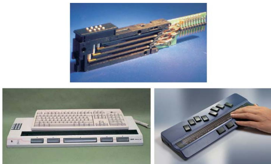
Figure 1.4: Current transitory Braille devices based on piezoelectric technology. "L"-shape Braille cell module with its corresponding electronics -top- with two examples of Braille devices on the market using such technology: Eco Plus-ONCE Braille keyboard [23] -bottom left-, and Active Braille 40 from ARC technology [24] -bottom right-.
