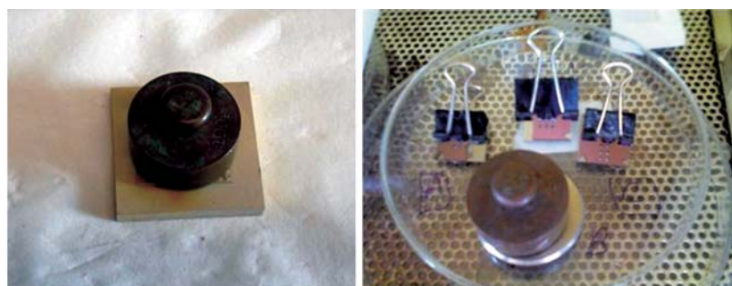
Figure 6.4: Stretching and crosslinking steps for the fabrication of the actuators.
