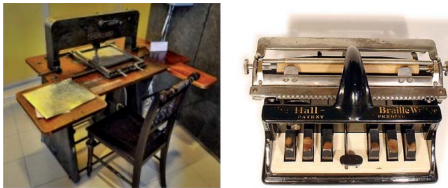
Figure 1.2: Braille machines from 19th century. German electromagnetic printer machine from 1938 [3] -left- and Frank H. Hall Braille personal typewriter machine [14] -right-.
