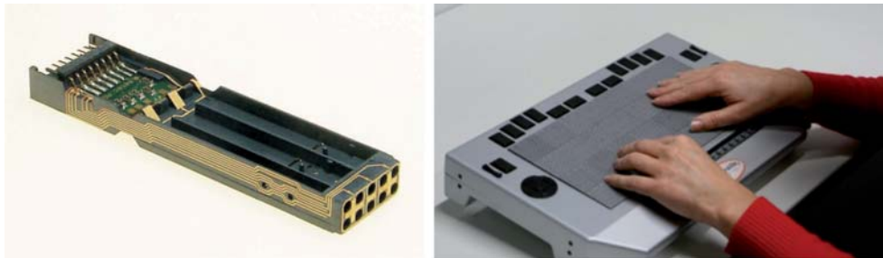
Figure 1.5: Novel piezo-driven technology for the fabrication of high density Braille device: Hyperbraille [29].
