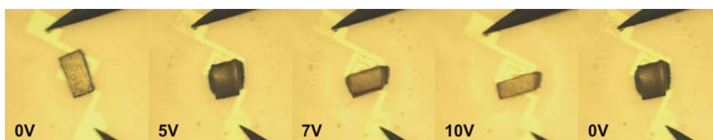
Figure 9.2: Example of permanent damage on a SCLCE sample due to an excess of voltage. Adapted from [238].
