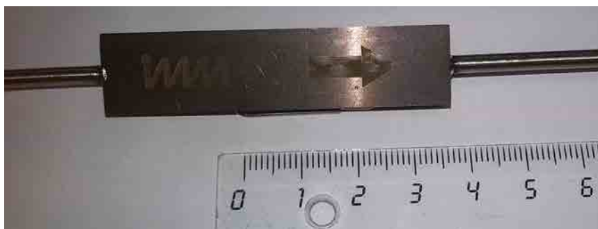
Figure 13.2: Welded platelets constituting a microreactor. The scale is shown in cm.
