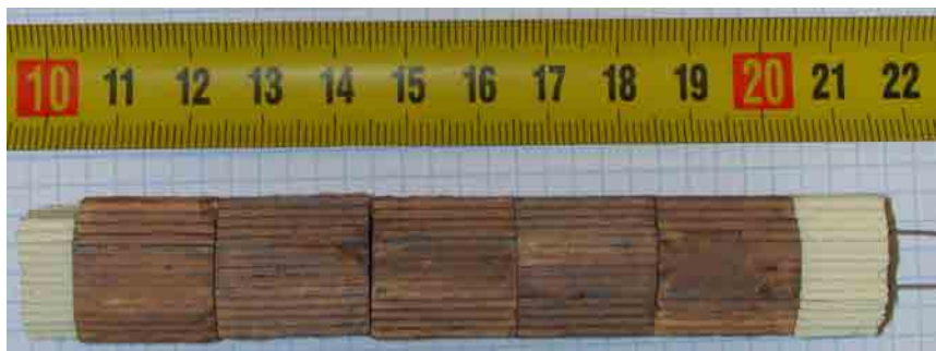
Figure 7.1: 1RhPd/ \text{CeO}_2 //Mon implemented in the membrane reactor. The scale is shown in cm.
