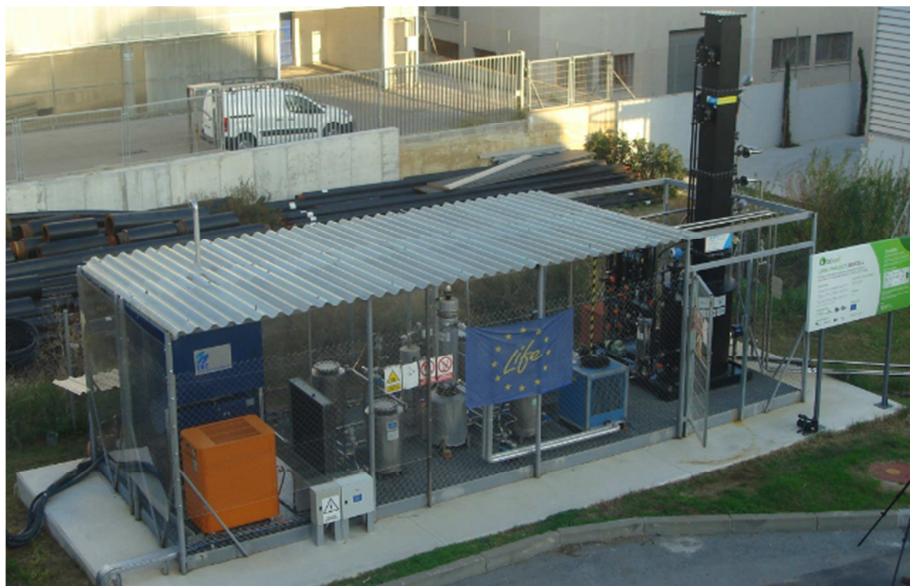
Figure 2.3. Sewage biogas powered Solid oxide Fuel Cell pilot plant
