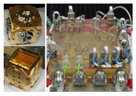
Figure 1.10: Left: electrode housing of the GRS. Credit: eLISA Consortium. Right: flight optical bench before integration into the LTP. The optical beams are applied into the optical bench by means of the fiber injector (green connectors). Credit: University of Glasgow and University of Birmingham.
