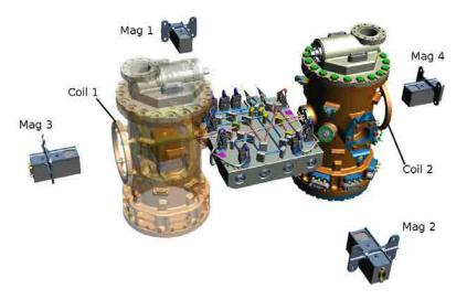
Figure 2.2: The payload of LISA Pathfinder with the four triaxial fluxgate magnetometers. Each of the electrode housings (cubic structures) inside the vacuum enclosure (the two cylindrical towers) encloses one TM at its center (solid gold cube).
