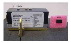
Figure 3.1: Fluxgate magnetometer used in LISA Pathfinder and AMR sensor proposed for eLISA. Size of the AMR is specified in Table 3.1.
