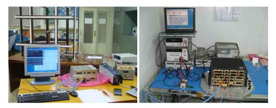
Figure 2.7: Test facility for measuring the range and uncertainty of the magnetic measurement subsystem. Left: engineering model test including the DMU and the magnetometer (in the center of the three-axis coil system). Right: test of the flight model DMU using simulated magnetometer readings.
