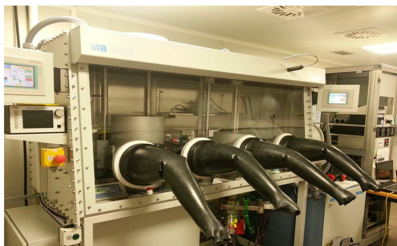
Figure 4.9 - Glovebox MB200B from MBraun with our home-made organic evaporator in 2012.
