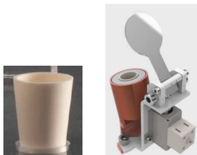
Figure 4.16 - Alumina boat (left). Alumina boat inside the heater system equipped with shutter (right).
