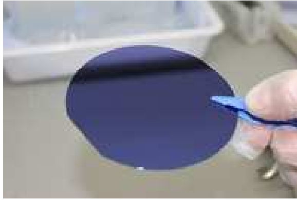
Figure A 2 - Silicon wafer with SiO 2 100-nm thick used as dielectric.
