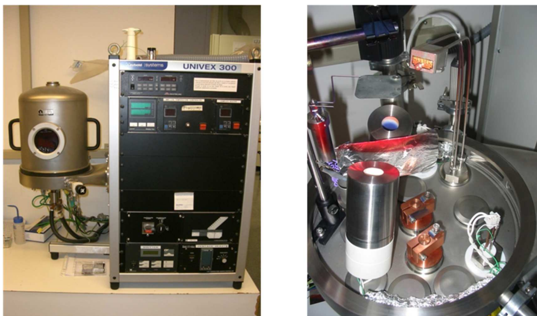
Figure 4.5 - Organic Evaporator UNIVEX 300 (left); Inside view of the chamber with two crucibles for p- and n-type respectively (right). In operation since 2006.
