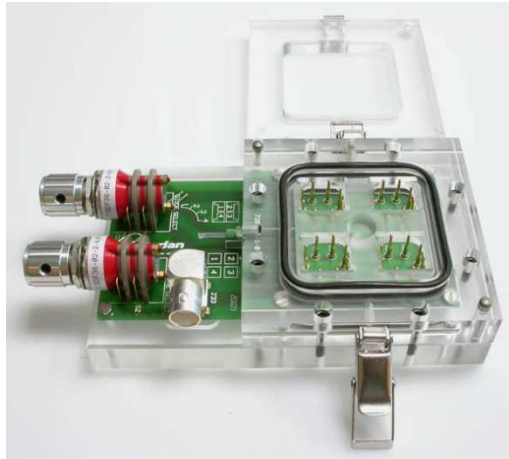
Figure 4.20 - Prototype to measure organic solar cells in nitrogen atmosphere.
