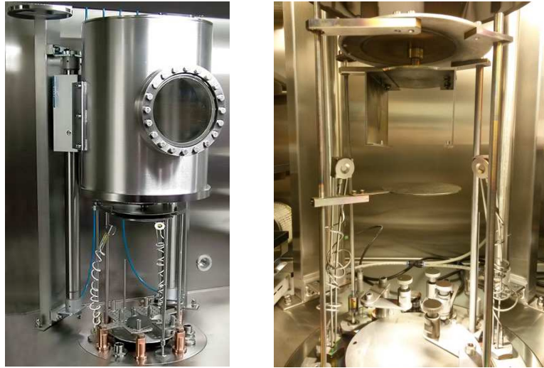
Figure 4.17 - MB-EcoVap (left); inside view with holder for mask (right).
