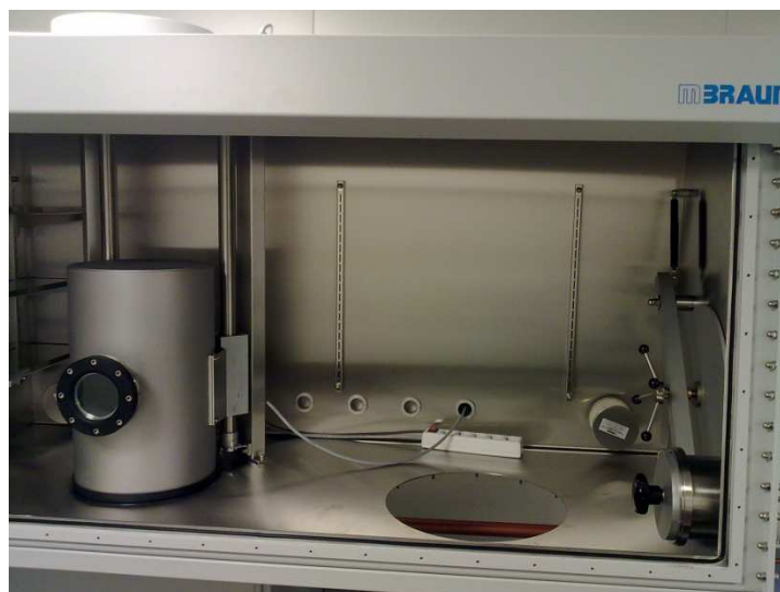
Figure 4.6 - Glovebox MB200B from MBraun with metal evaporator in 2010, before the installation of organic evaporator.
