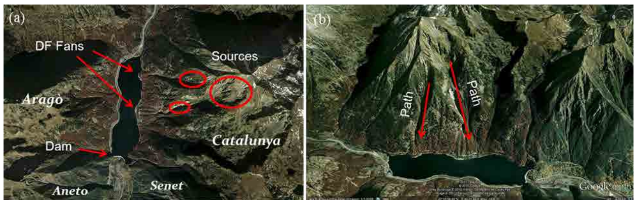
Figure 1.10. Baserca Reservoir, Spain: a) descriptive map of the reservoir with sources and fans of debris flows (DF) (aerial photo of Institut Cartografic de Catalunya, 2011); b) oblique image of the spot with the debris-flows paths (Google Earth, 2009).
