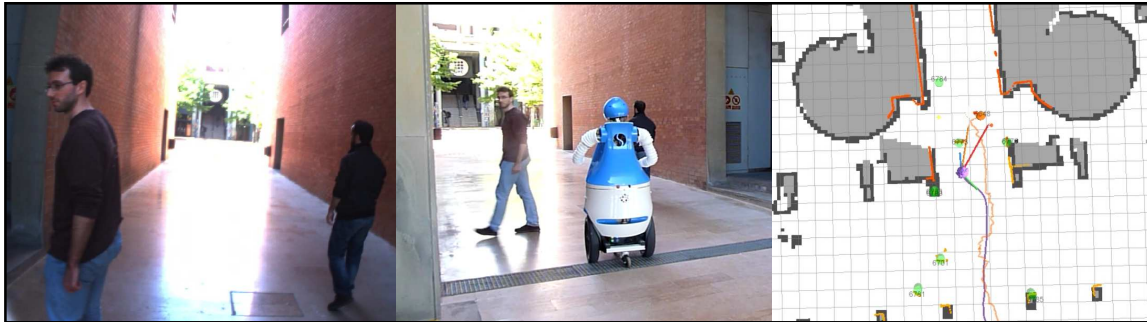
Figure 3.9: Example of a real robot experiment. The left image corresponds to the robot camera. On the center of the image Dabo is accompanying a person to her desired goal while navigating in a urban environment. The right image corresponds to the robot GUI, built on ROS architecture. Green cylinders correspond to persons' detections and the orange cylinder corresponds to the target to be accompanied.
