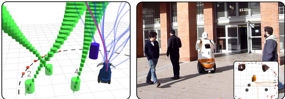
Figure 7.1: Robot navigation. Left: Simulation environment in a space \times time , where people are plotted as green cylinders and their predictions are drawn in the z axis, which corresponds to time. The tree of paths calculated by the robot appears in blue and the best path is a red line. Right: Example of robot navigation in a urban environment, the BRL. in a simplified visualization of the environment.
