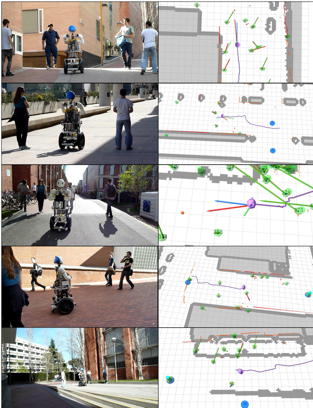
Figure 5.5: Real experiments. Left: some pictures of the social-aware approach navigating in the BRL. Right: their corresponding sensor information, virtual forces and trajectories in the robot GUI using ROS.
