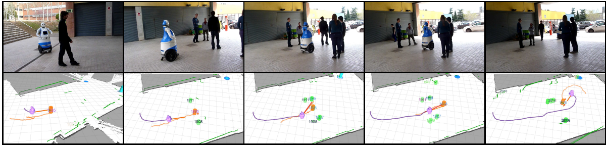
Figure 6.10: Real-life experiments. A single robot companion experiment. Top: Dabo accompanying a person to a desired goal. Bottom: The same scene using the system interface.
