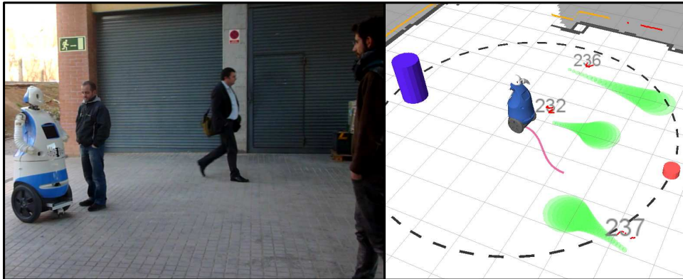
Figure 4.2: Urban environment. Scene corresponding to the FME, where part of the experiments were carried out. Prediction position covariances are drawn as green ellipses projected and superposed in the plane.
