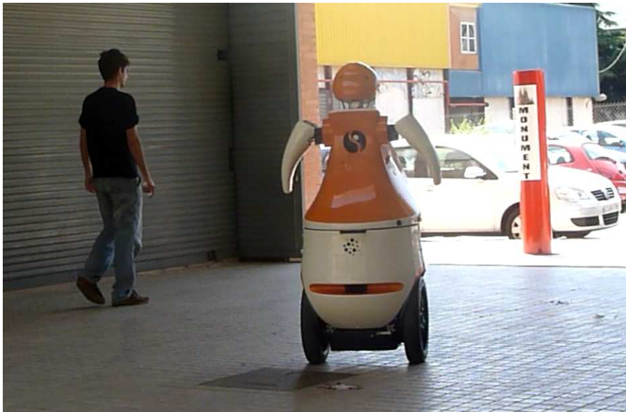
Figure 3.1: Example of a destination in the environment. In this controlled setting, the red pylon represents a scene destination that both the robot and the volunteer try to reach. We use the BHMIP to infer the most expectable destination of the person.
