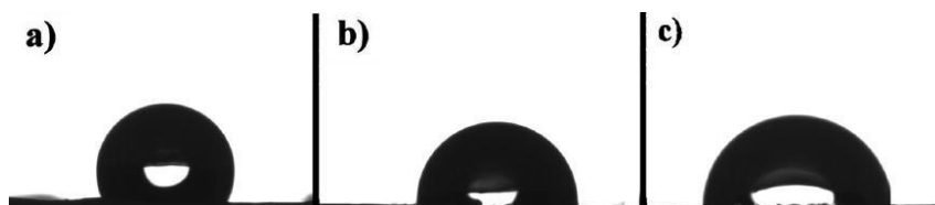
Figure 1.2.6. Wettability changes of the P4 membrane (a) before irradiation, (b) after UV irradiation at 365 nm, and (c) after UV irradiation at 365 nm followed by additional irradiation at 245 nm.
