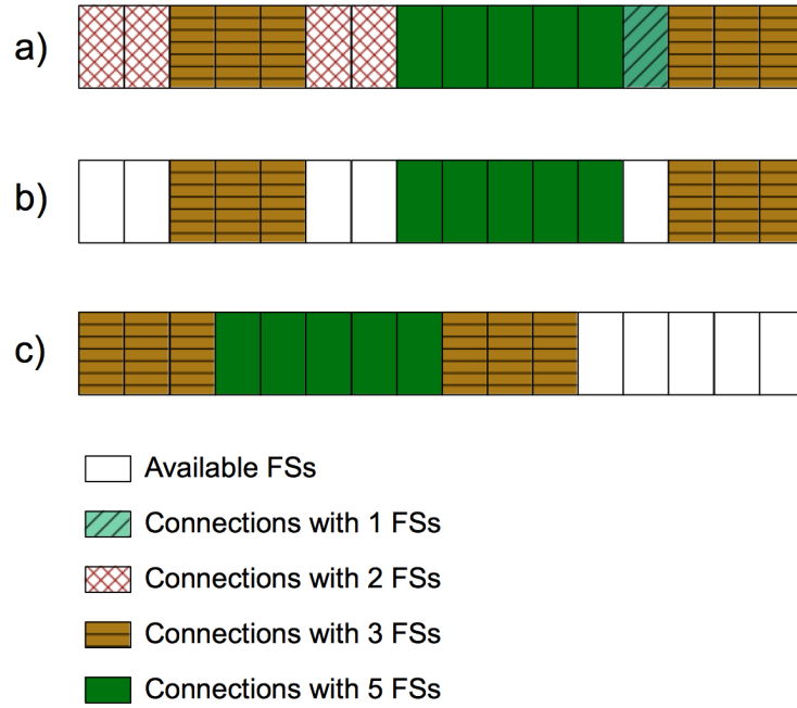
Figure 3.5: The diagram shows a) original link state before connections termination, b) spectrum fragmented link after connections termination and c) link state after defragmentation
