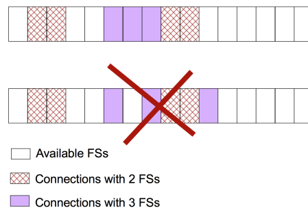
Figure 2.6: The diagram shows a) connections with contiguous allocated FSs and b) one connection has non-contiguous allocated FSs, this is not possible in an EON
