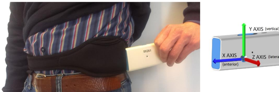
Figure 4.9: The inertial system prototype (9x2, Version 6) positioned in a neoprene belt
