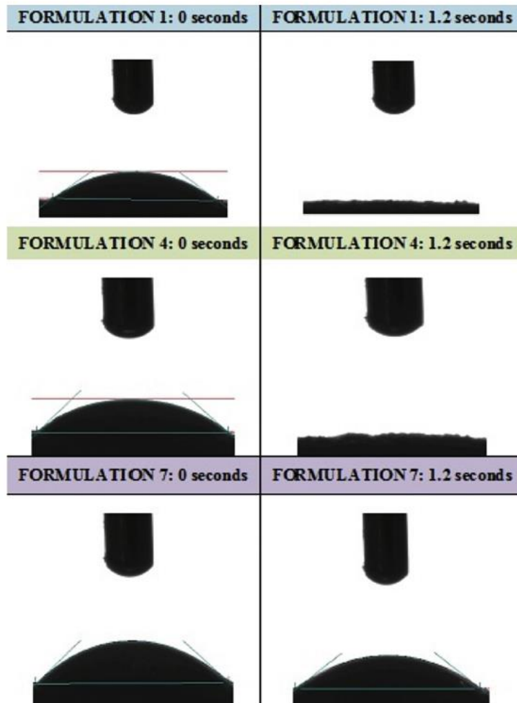
Fig. 4. Contact angles of formulations 1, 4 and 7 in water at t=0 and 1.2 s.
