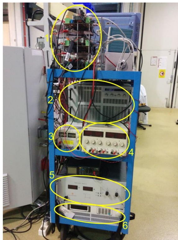
Fig. 5.23. Front view of the cart containing the three BBCOFs (1), the electronic load (2), a DC source for the cooling fans (3), a DC source for the control board (4), the DC source 1 (5) and the DC source 2 (6).
