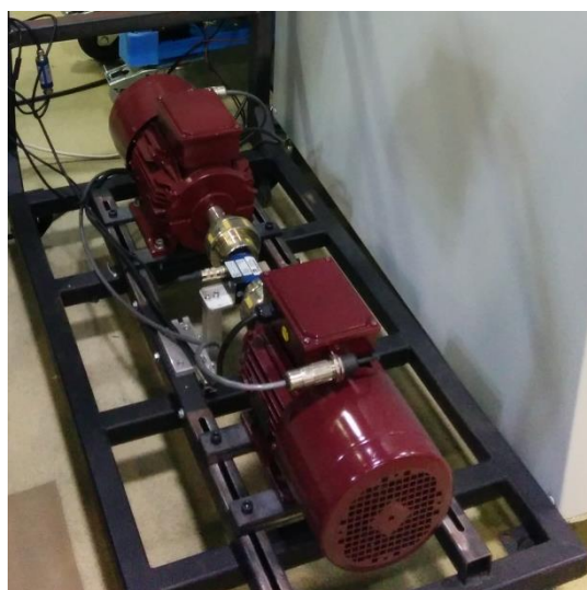
Fig. 5.21. Detailed view of the two mechanically coupled PMSMs.
