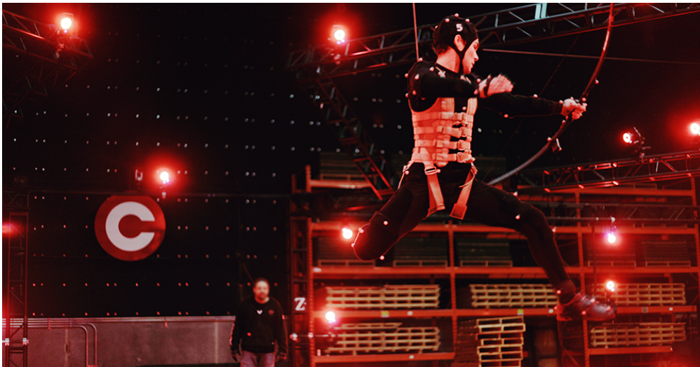
Figure 2.1: An actor dressed in a suit with markers being captured while performing a shoot with a bow. [The Capture Lab, 2015]
