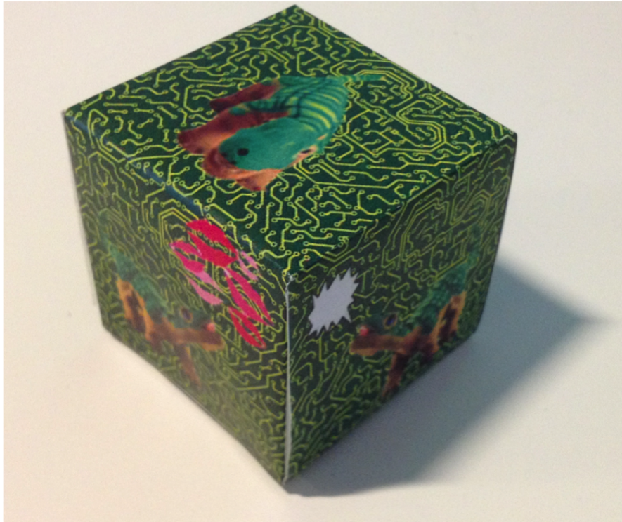
Figure 5.19: Physical cube built to drive Vleo. Their faces are illustrated with Pleo images that represents the actions that Vleo can perform.
