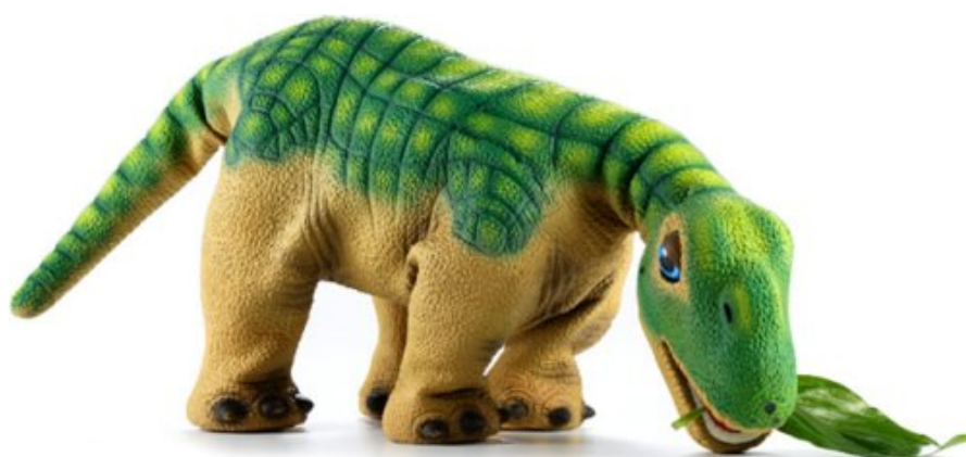
Figure 5.13: Pleo "eating". When you buy Pleo, it comes with an electronic dna green leaf. If you call your Pleo and show it the leaf, it will come and get close to the leaf and sniff it (actually at this moment it is watching the leaf with a small camera on his nose) then finally bite the leaf and a crunch sound will be heard.
