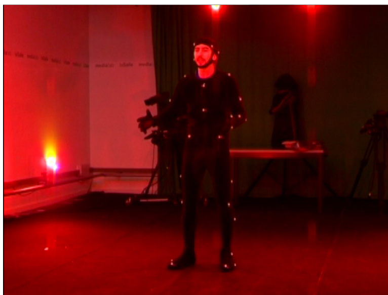
Figure 4.5: Set-up of the recording session. An optical motion capture system with 24 infrared cameras, a clip-on wireless microphone, and a videocamera (not in the image). The actor is wearing a black motion capture suit with reflective markers.
