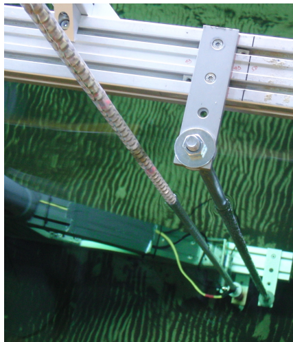
Fig. 3.9 Photograph of the cylinders in tandem configuration, To the right is a rigid leading cylinder, whereas the on the left is the flexible, densely instrumented trailing cylinder with mass ratio m^* = 2.7
