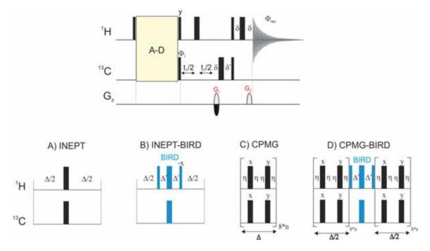
Figure 17: Several 2D non-refocused HSQMBC pulse schemes to obtain heteronuclear long-range correlation spectra ( $\Delta$ =1/[2<sup>n</sup>/<sub>CH</sub>]). The initial transfer step is: A) a basic INEPT, B) an INEPT-BIRD block ( $\Delta'$ =1/[2<sup>1</sup>/<sub>CH</sub>]); C) a CPMG XY-16 super cycle consisting of simultaneous <sup>1</sup>H and <sup>13</sup>C pulses applied at intervals 2 $\eta$ ; D) a CPMG-BIRD element combining the features described in B and C.
