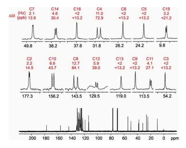
Figure S3: (Bottom) 150.9 MHz Broadband heterodecoupled  $^{13}$ C NMR spectrum of racemic compound **1** and *R*-PA; (top) expanded multiplets to show individual signal splitting (in Hz and ppb) due to the enantiodifferenation.
