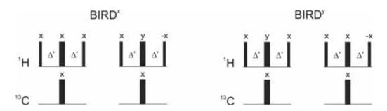
Figure 3: Different implementations of the BIRD<sup>x</sup> (right) and BIRD<sup>y</sup> (left) NMR building blocks. Δ' is adjusted according to  $1/(2^1 J_{CH})$ .
