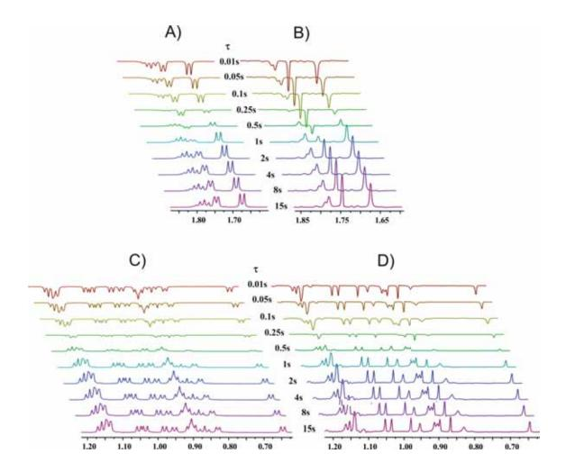
**Figure S4**: IR and HOBS-IR experiments of the selected aliphatic areas described in Fig. S3. The homodecoupling conditions in B and D were the same as described in Fig. S3 and the experimental  $T_1$  values are shown in Table S1.
