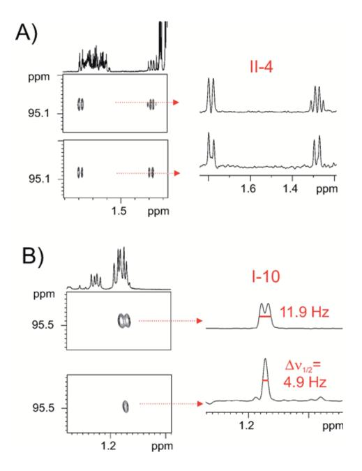
Figure S14: (top) Conventional and (bottom) broadband homodecoupled HSQC A) II-4 (diastereotopic  $CH_2$ ) and B) I-10 ( $CH_3$ ) cross peaks. 1D slices on the right allow to compare the relative sensitivity, the multiplet simplification and the experimental line widths achieved in both experiments.
