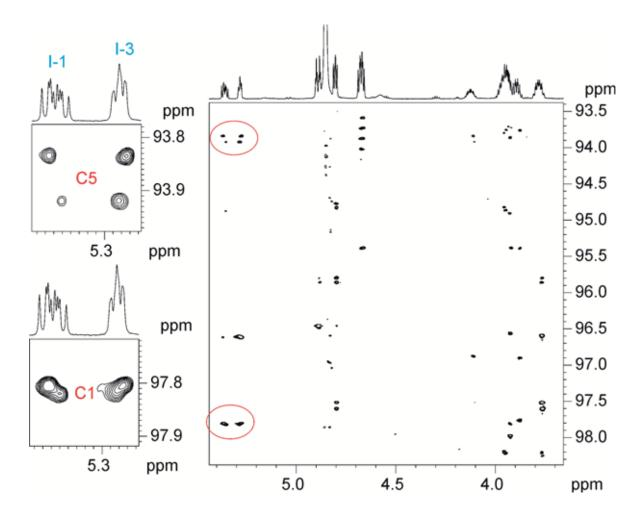
Figure S5: Spectral-aliased 2D <sup>1</sup>H-<sup>13</sup>C HOBS-HSQMBC spectrum acquired with SW(<sup>13</sup>C)=5 ppm. Note the key long-range H3-C1, H1-C5 and H3-C5 correlations in the expansions.
