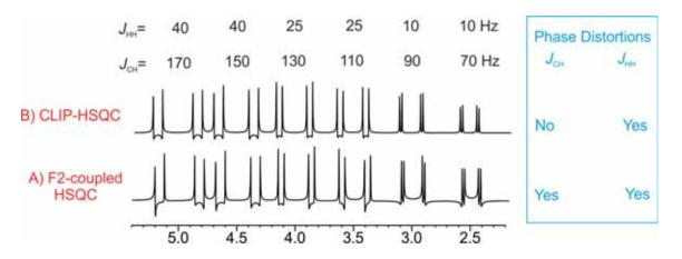
Figure 14: Simulated 1D spectra showing the phase peak distortion effects in 140-Hz optimized A) F2-heterocoupled HSQC and B) CLIP-HSQC spectra. Six protons belonging to three different diastereotopic CH<sub>2</sub> groups have been simulated with a wide range of  $J_{HH}$  and  $^1J_{CH}$  values, as shown in the upper part.
