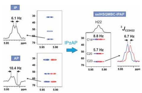
Figure 20: selHSQMBC-IPAP experiments after selective excitation of the olefinic H22 proton in strychnine [2]. The acquired A) IP and B) AP datasets are added/subtracted to provide C) separate  $\alpha/\beta$  subspectra. The relative displacement between  $\alpha/\beta$  cross-peaks along the F2 dimension provides a direct measurement of  $^{n}J_{CH}$  without any posterior analysis.
