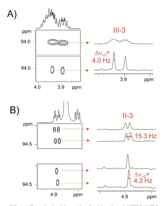
Figure S13: (top) Conventional and (bottom) broadband homodecoupled HSQC A) III-3 and B) II-3 cross peaks. 1D slices on the right allow to compare the relative sensitivity, the multiplet simplification and the experimental line widths achieved in both experiments.
