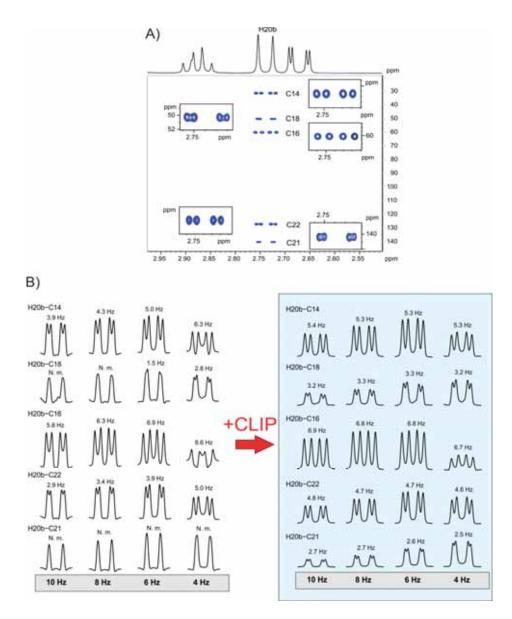
Figure 19: A) 2D CLIP-selHSQMBC spectrum of strychnine [2] after pulsing on H20b with a 20 ms Gaussian-shaped  $180^{\circ}$  <sup>1</sup>H pulse. The inter-pulse delay  $\Delta$  was optimized to 62.5 ms (corresponding to  $^{\circ}J_{CH} = 8$  Hz). B) Direct extraction of  $^{\circ}J_{CH}$  can be made from pure in-phase cross-peaks, independent of experiment optimization (from 4 to 10 Hz).
