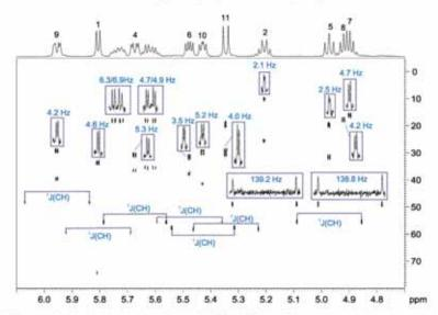
Fig. 5. In-phase HOBS-HSQMBC spectra of cyclosporine showing how the value of J(CH) for all direct and long-range cross-peaks can be extracted directly from the analysis of the clean doublet along the detected dimension (see the extracted value in each individual 1D inset). Note that only the AB spin system (protons resonating at 5.62 and 5.73 ppm) appears as a double of doublets due to their mutual J(HH).
