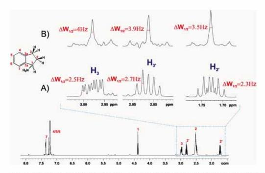
**Figure S1:** Experimental linewidths measured a 50mM (*RS*)-aminoindan sample dissolved in CDCl<sub>3</sub>: A) conventional  $^{1}H$  and B) homodecoupled  $^{1}H$  SPFGE spectra after individual selection of each proton. All data were processed without any window function. The homodecoupling conditions in B) were: a 20 ms Gaussian shaped  $180^{\circ}$   $^{1}H$  pulse,  $\Delta$ =19 ms, n=15 and AQ=568 ms.
