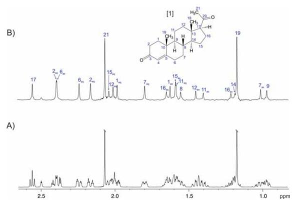
**Figure 1**: 600 MHz A) conventional and B) broadband homodecoupled 1D  $^{1}$ H NMR spectra of the steroid progesterone [1] in DMSO-d<sub>6</sub>. Note how all simplified singlet resonances at their chemical shift frequencies can be distinguished in the pure shift spectrum.
