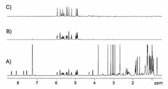
Figure S1: (A) <sup>1</sup>H spectrum of cyclosporine; B) Band-selective spectrum acquired with the single-pulsed-field gradient echo (SPFGE) sequence using a semiselective RE-BURP-shaped 180° <sup>1</sup>H pulse of 5 ms; and C) 1D HOBS spectra acquired with the pulse sequence of Fig. 1 using a 5ms REBURP-shaped pulse.
