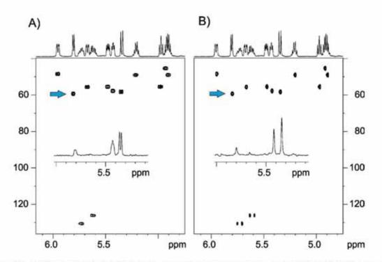
Figure S7: A) Conventional and B) fully homo- and heteronuclear decoupled HOBS-HSQC spectra of cyclosporine obtained using the non-refocused version of Fig. S6B with the same experimental conditions as described in Fig. 4. Note the J(HH) doublet splitting of the two olefinic AB protons. More details can be found in the experimental section.
