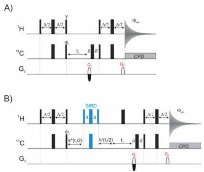
Figure 15: Several pulse schemes to achieve F1-heterocoupled HSQC spectra: A) F1-coupled HSQC, and B) F1-coupled BIRD-HSQC. The interpulse delay in INEPT and BIRD elements are optimized according to  $\Delta$ =1/(2 $^{1}J_{\text{CH}}$ ). A minimum two-step phase cycling is executed with  $\Phi_{1}$ =x,-x and  $\Phi_{\text{rec}}$ = x,-x, all other unlabeled pulses are from the x-axis. Gradients  $G_{1}$  and  $G_{2}$  are used for coherence selection using E/A ( $G_{1}$ :  $G_{2}$ =±80:20.1).
