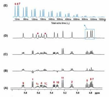
Fig. 3. Comparison of 1D (A) conventional <sup>1</sup>H, (B) CPMG, (C) PROJECT, and (D) HOBS-PROJECT spectra of cyclosporine acquired with a total echo time of  $\tau_e$  = 156 ms (m = 26 and  $\tau'$  = 1.5 ms). All spectra were collected under the same experimental conditions as described in Fig. 2 and are plotted at the same absolute vertical scale. (E) Signal  $T_2$  decays for the H5, H8 and H7 protons in the HOBS-PROJECT experiment.
