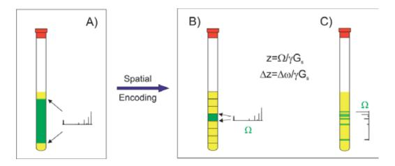
**Figure 5**: Different strategies to induce spatial selection along the *z*-axis of a NMR tube: A) Standard excitation/detection over the entire coil; B) Single-slice selection; C) Frequency-selective spatial selection.
