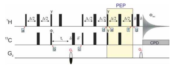
Figure 11:  $^{1}\text{H}-^{13}\text{C}$  HSQC-PEP pulse sequence using the E/A method.  $\Delta=1/(2^{1}J_{\text{CH}})$ ,  $\Delta_{1}=\Delta$  for CH multiplicities,  $\Delta_{1}=1/(4^{1}J_{\text{CH}})$  for all multiplicities. A basic two-step phase cycling is executed with  $\Phi_{1}=x$ ,-x and  $\Phi_{\text{rec}}=x$ ,-x. Coherence selection is performed by the gradient pair  $G_{1}:G_{2}$  ( $\pm 80:20.1$ ) using the echo-antiecho protocol.
