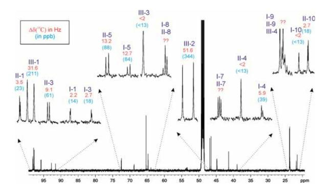
Figure S1: 150.62 MHz 1D <sup>13</sup>C NMR spectrum of the mixture. Expanded areas shows the chemical shift differences (in Hz and ppb) observed for analog carbons in the mixture of the diastereoisomers Ia/Ib, IIa/IIb and IIIa/IIIb.
