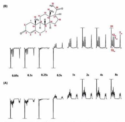
Fig. 4. Experimental decays in (A) IR and (B) HOBS-IR experiments of all protons resonating in the region 1.8-2.1 ppm in progesterone. All spectra are plotted in the same absolute vertical scale. Homodeocupling was achieved using the detection scheme described in Fig. 1A with a 20 ms REBURP 180° pulse, 4 = 12.37 ms, AQ = 569 ms and n = 23.
