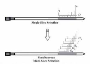
Figure 1. Schematic representation of a conventional single-slice pulse sequence compared to simultaneous multi-slice selection by a multiple-frequency pulse modulated according to different offset frequencies ( $\Omega_1 \dots \Omega_k$ ). A methodology is described that avoids the simultaneous excitation of mutually J-coupled spins within the same z slice.
