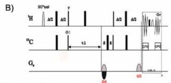
Figure S6: A) 1D HOBS detection scheme to perform simultaneous broadband homo- and heteronuclear decoupling. Heteronuclear Decoupling (CPD) is only applied during data writing and it is switch off during the application of the gradient-based inversion elements; B) Pulse scheme of the fully homo- and heteronuclear decoupled HOBS-HSQC experiment.
