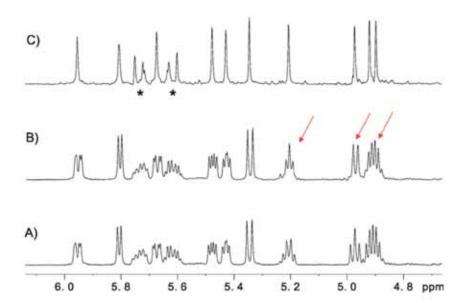
Figure S3: Expanded  $H_{\alpha}$  region corresponding to the spectra of Fig. S2. The selective decoupling of the NH region in B only simplifies the  $H_{\alpha}$  protons with a resolved J(NH-  $H_{\alpha}$ ) coupling (see arrows). Note that other couplings between  $H_{\alpha}$  and other side-chain  $H_{\beta}$  protons are not affected. In C) all couplings are collapsed except the active J(HH) of the olefinic AB spin system (marked with asterisks).
