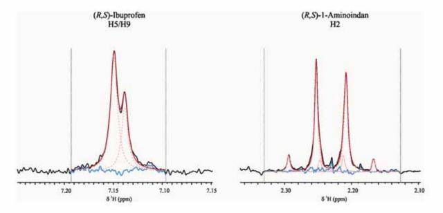
**Figure S5:** Examples of line fitting achieved for the singlets obtained from the HOBS spectra after selection the H5/H9 protons of (*R*,*S*)-ibuprofen (35:65) and H2' in (*RS*)-1-aminoindan samples. The experimental results are listed in Table S1.
