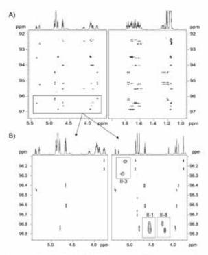
Figure 4. A) Spectral-aliased HSQC-TOCSY spectrum of the mixture acquired with SW("IC) = 5 ppm; B) Expansions to compare the spectral-aliased HOBS-HSQC vs. HOBS-HSQC-TOCSY spectra on region A. In addition to proper assignments, note that relayed cross-peaks can visualize splitting that is not observed with direct correlations.
