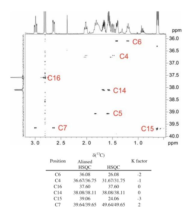
Figure S10: Chemical shifts in aliased and conventional 2D psHSQCsi spectra. Experimental parameters in the indirect dimension: carrier frequency= 38.0 ppm and  $^{13}$ C spectral width= 5 ppm.
