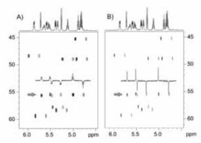
Figure 4. A) Regular, and B) HOBS spectra of the non-refocused F2 coupled  $^{1}\text{H-}^{12}\text{C}$  HSQC experiment of **I**. The interpulse delays were optimised to 145 Hz. Two scans were collected for each one of the 64  $t_1$  increments of 2 K complex data points. Homodecoupling was achieved using n=50,  $\Delta=5.7$  ms. AQ=570 ms. sw=1800 Hz and a REBURP 180° pulse of 5 ms. The experimental time for each 2D spectrum was of 5 min.
