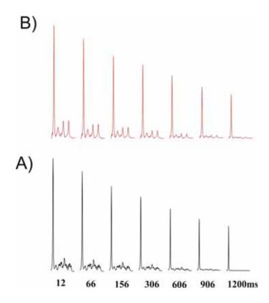
**Figure S6**: Stacked plot of the 600 MHz 1D spectra of progesterone acquired with the A) PROJECT and B) HOBS-PROJECT experiments using the conditions described in experimental section and Fig. S5. The individual  $T_2$  values can be found in Table S2.
