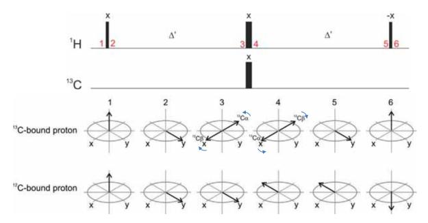
**Figure 4**: Pulse sequence of the BIRD<sup>9</sup> element used to invert the magnetization of <sup>12</sup>C-bound protons while leaving the magnetization of <sup>13</sup>C-bound protons essentially unaffected. The fates of the <sup>13</sup>C- and <sup>12</sup>C-bound protons magnetizations are shown in the vector representation. The spin state of the bound <sup>13</sup>C nucleus is also indicated.
