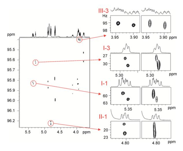
Figure S2: (left) 2D HOBS-HSQC spectrum of the region I acquired with a SW(<sup>13</sup>C)=1 ppm. (right) Comparison of some expanded cross-peaks in HOBS-HSQC spectra acquired with SW(<sup>13</sup>C)=1 and 5 ppm, respectively.
