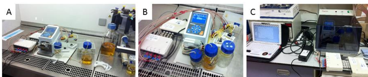
Figure 5.1. Continuous flow experiment preparation. (A) Connection of all the components inside a biosafety cabinet. (B) Assembly of the platform, bottles and peristaltic pump on the incubator tray. (C) Perform the software to connect by Bluetooth the impedance analyser with the laptop and record the data wireless.
