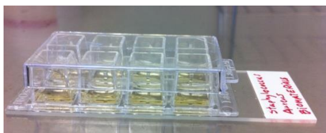
Figure 7.4. 8-well chamber slide with bacteria suspended in TSB medium for testing different concentrations of bacitracin attached on the modified surface.
