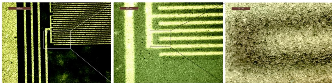
Figure 6.11. Presence of biofilm developed in the flow chamber at the end of the experiment. The image shows the bacterial structure over the interdigitated microelectrode (IDuE) in a detailed pseudo-3D image carried out with Differential Interference Contrast (DIC). Magnifications: (A) 5X; (B) 20X; (C) 100X.
