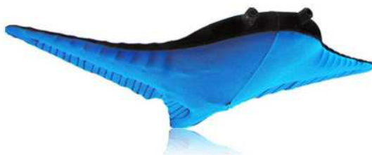
Figure 2.14: Subsea Glider with Fin Ray Effect.
