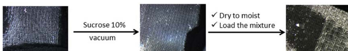
Figure 4.5-2: Microporous elastomeric membranes pre-conditioning protocol. The proposed elastomeric membranes were highly hydrophobic as it can be observed in (Figure 4.5-3a). The first attempt to facilitate the penetration of the aqueous mixture inside the elastomeric membranes pores was to fill the pores with PBS with the aim that this facilitates the diffusion of the mixture. Firstly the membranes were sterilized with EtOH 70 % and carefully dried. PBS was forced to penetrate into the pores of the elastomeric membrane pores using vacuum, and then it was substituted by sucrose 10 % to avoid RAD16-I peptide gel. Once the sucrose 10 % were filling the pores the elastomeric membrane was dried to moist. At this step, the membranes were prepared for the loading of cells + peptide mixture.
