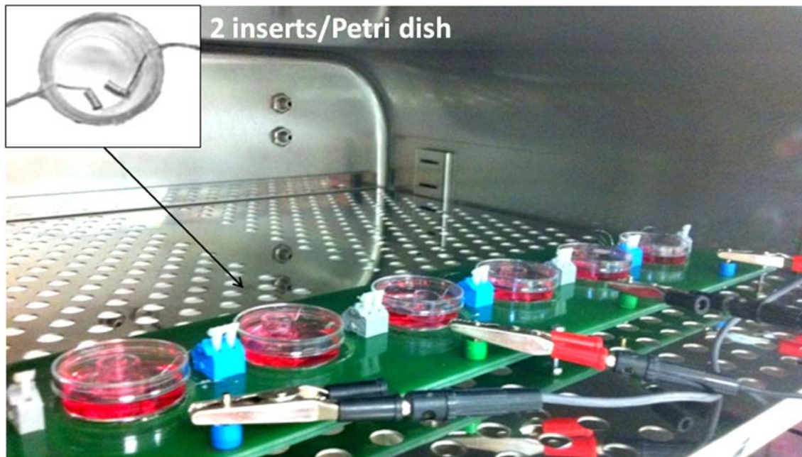
Figure 3.4-1: The electrical stimulation set-up inside the cell culture incubator. The Printed Circuit Board (PCB) (in green), cultures plates with media and detail of an insert with the stimulation electrodes (left top).
