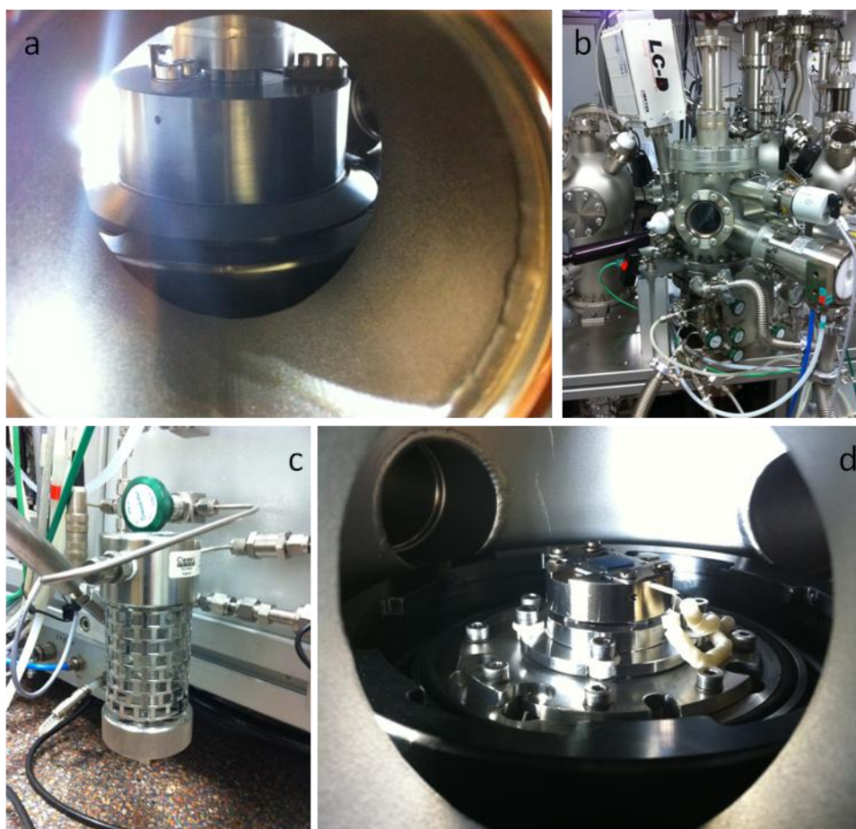
Figure 22 (a) reaction chamber closed. (b) External view of the reaction chamber. (c) Vaporizer. (d) Detail of the sample inside the reaction chamber.
