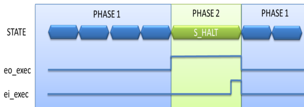
Figure A.2: Handshake sequencer signals for change of the operation mode
