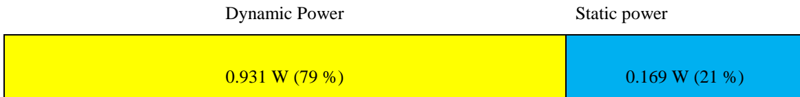
Figure 5.12: Power consumption of fully connected SNAVA 10 x 10
