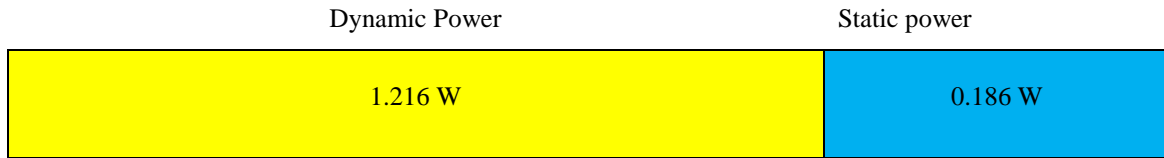
Figure 5.22: Power consumption of SNAVA+ with 10x10 PE array size and 99 synapses per PE unit
