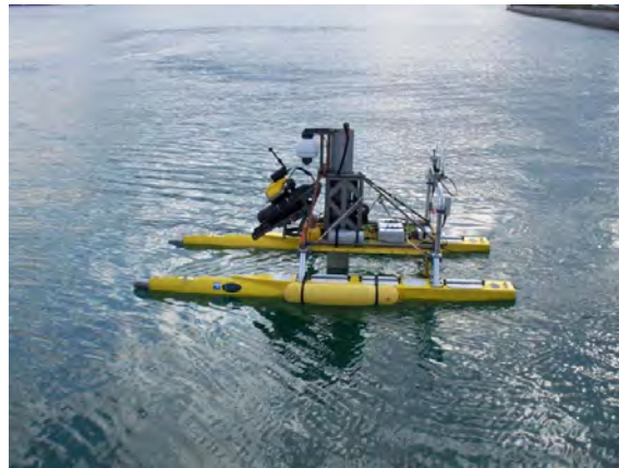
Figure 6.11: ASV equipped with the Blueview P900-130 FLS used in the Marina Marciana experiment. Image credit: CMRE.
