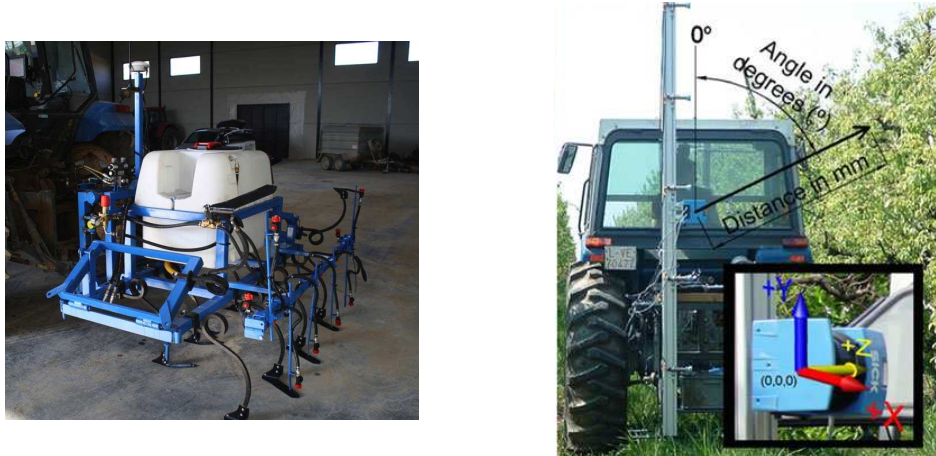
Fig. 1.3. (a) Weed control prototype [34]; (b) LAI prediction by using LIDAR sensors mounted on a tractor [36].
