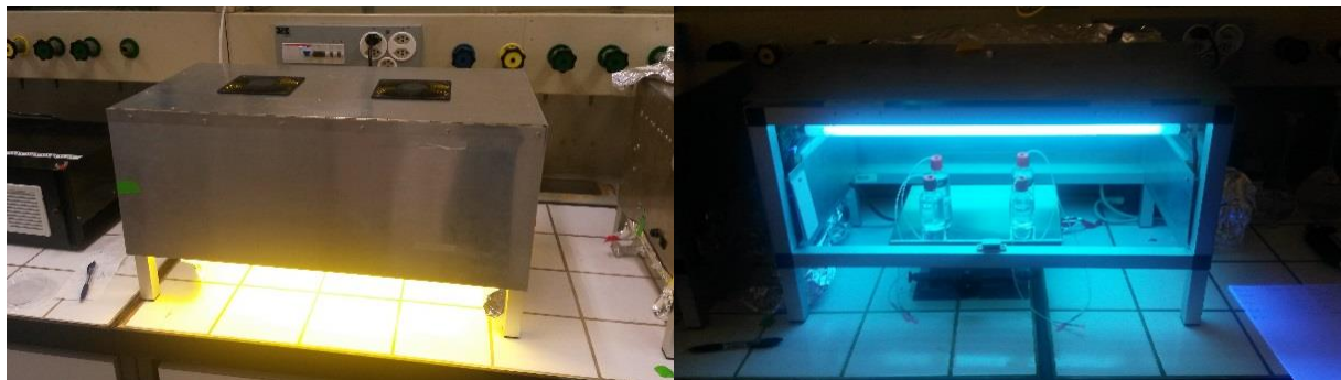
Figure 4.1.4: The light apparatus bearing the monochromatic and visible light lamps. On the left, the yellow light at work and on the right, the actinic backlight. The spatial distribution of the reactors is also visible.
