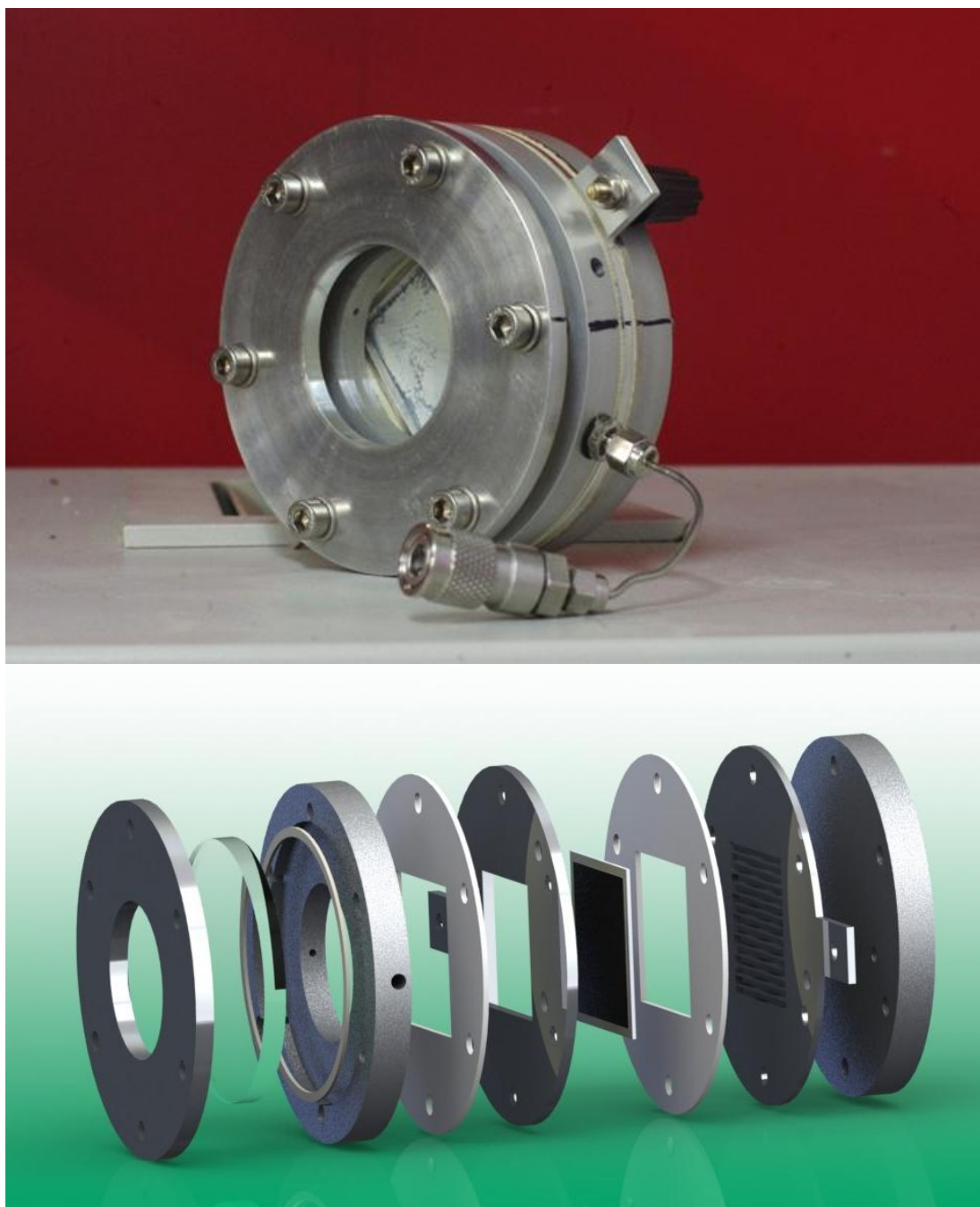
Figure 6-2. PEC cell design project (bottom) and assembled cell ready for testing (top)
