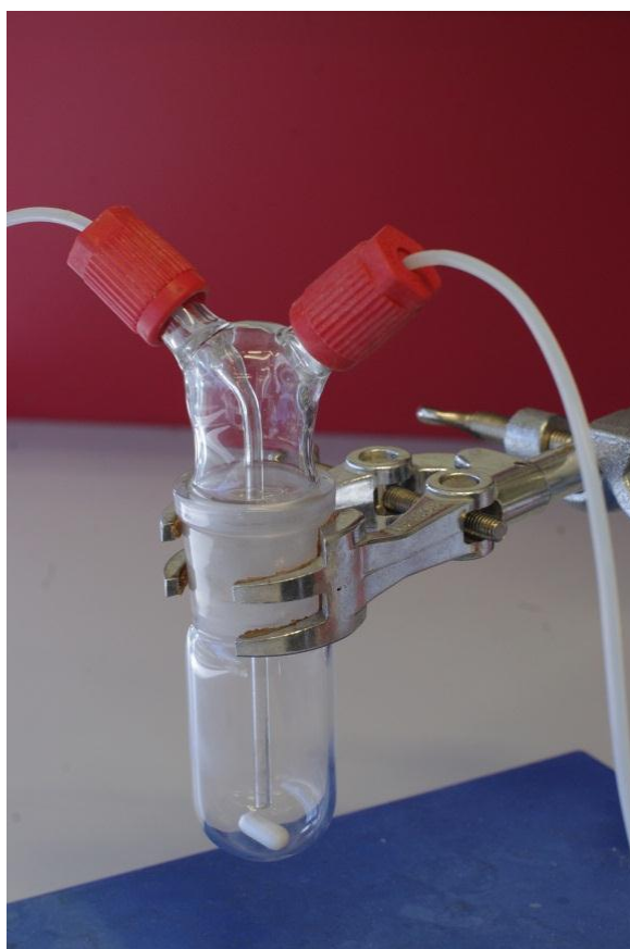
Figure 2-6. Continuous liquid phase (slurry) photocatalytic reactor
